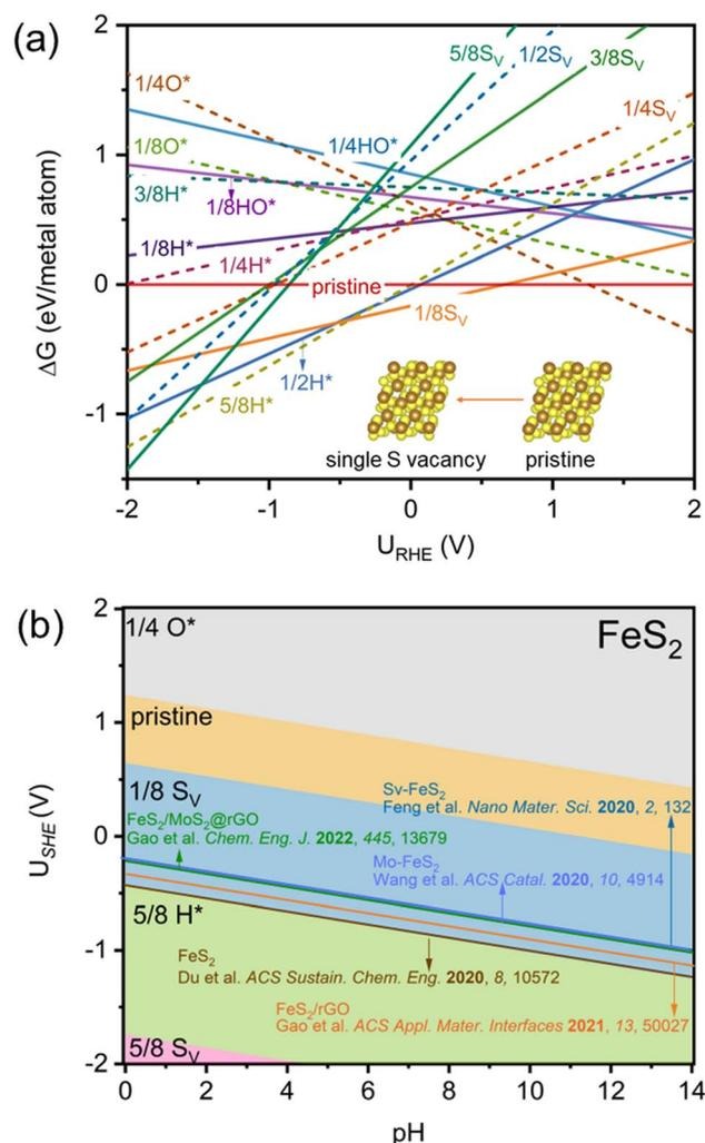
Fig. 2 Calculated (a) 1D and (b) 2D surface Pourbaix diagrams of  $\text{FeS}_2(111)$  considering different coverages of  $\text{S}_\text{V}$ ,  $\text{O}^*$ ,  $\text{H}^*$ , and  $\text{HO}^*$ . The experimental potentials at the highest faradaic efficiencies of reported  $\text{FeS}_2$ -based catalysts are plotted for a direct comparison. These experimental data were extracted from ref. 18–20, 22 and 27.
