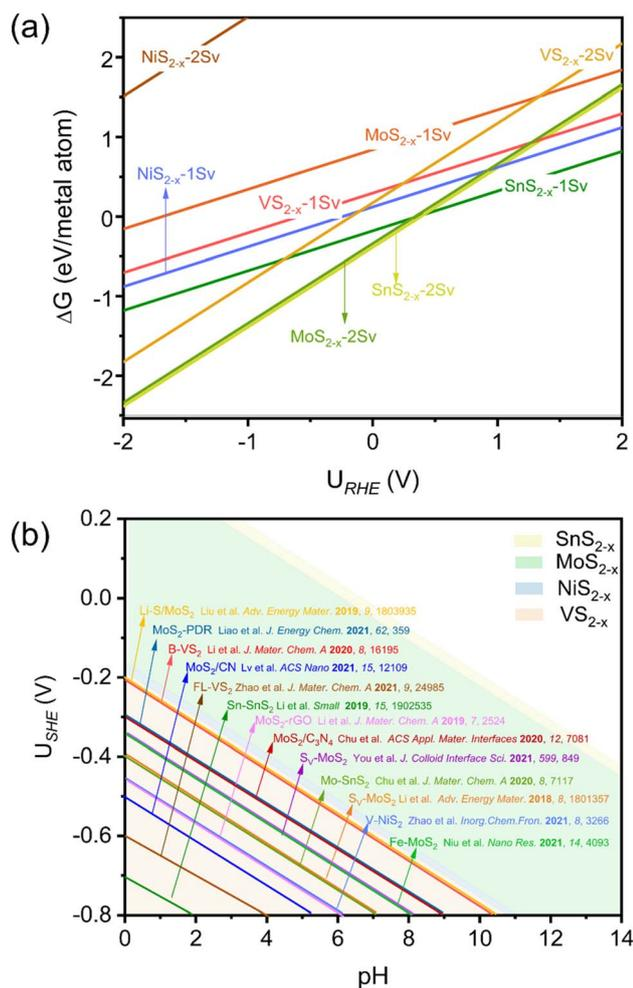
Fig. 5 (a) 1D surface Pourbaix diagrams of different transition metal disulfide (TMS<sub>2</sub>) surfaces. (b) 2D surface Pourbaix diagram of S<sub>v</sub> formation as a function of pH and potential. The color-coded segments demarcate the potential windows of S<sub>v</sub> generation on the respective instances of TMS<sub>2</sub>. The reported experimental operating potentials at their highest NH<sub>3</sub> faradaic efficiencies are drawn on the diagram.<sup>23–25,28,46–54</sup>
