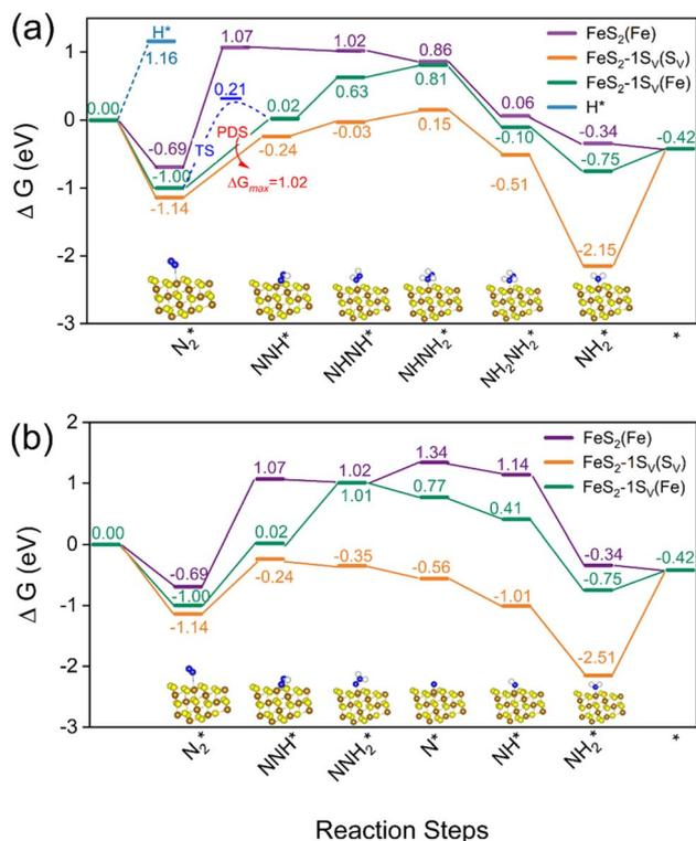
Fig. 3 Calculated Gibbs free energy diagrams of ENRR over  $\text{FeS}_2(111)$  and  $\text{FeS}_{2-x}(111)\text{-}1\text{S}_V$  surfaces. (a) and (b) demonstrate the energy profiles through the alternating and distal pathways, respectively. The insets show the optimized geometries of the key reaction intermediates. Brown, yellow, blue, and white spheres represent Fe, S, N, and H, respectively.
