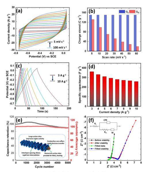
Fig. 2 Electrochemical study of heterostructured  $Sb_2S_3/MoS_2$ . (a) CV curves of  $Sb_2S_3/MoS_2$ , (b) surface and diffusive charges stored at different scan rates for  $Sb_2S_3/MoS_2$ , (c) GCD curves of  $Sb_2S_3/MoS_2$ , (d) specific capacitance of  $Sb_2S_3/MoS_2$ , (e) cycling stability of  $Sb_2S_3/MoS_2$  and (f) Nyquist plots before and after  $Sb_2S_3/MoS_2$  stability tests (inset: fitted circuit).
