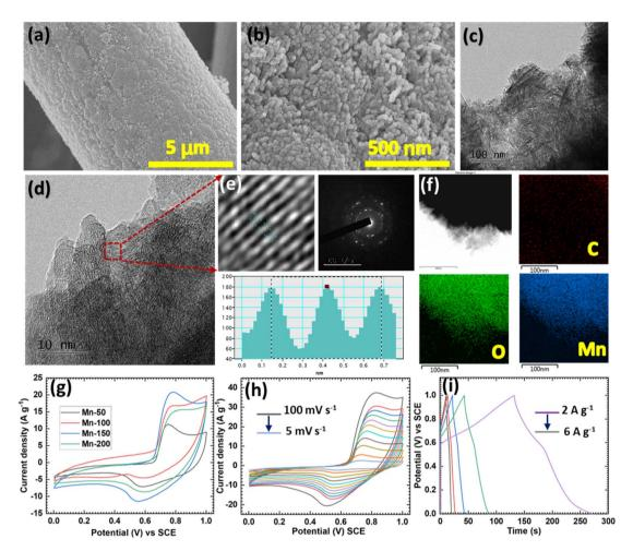
Fig. 3 (a and b) SEM images of MnO<sub>2</sub> and (c-e) TEM images and (f) elemental mapping of MnO<sub>2</sub> (Mn-150 sample). (g) Comparative CV curves for the Mn series of electrodes. (h) CV curves at different scan rates and (i) GCD curves at different current densities for the Mn-150 electrode.
