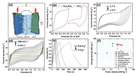
Fig. 4 Electrochemical study of AIHC. (a) Schematic presentation of ammonium-ion storage. (b) CV curves of  $MnO_2$  and  $Sb_2S_3/MoS_2$  in different voltage windows, (c) CV curves at different potential windows, (d) CV curves at various scan rates, (e) GCD curves at different current densities, and (f) Ragone plot comparison with materials reported in the available literature.
