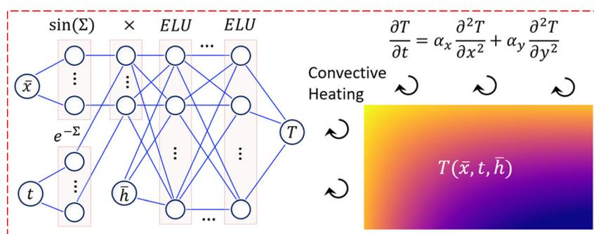
Fig. 2 Application of ML in the prediction of temperature using spacial and temporal parameters as independent variables in transient convection of a porous medium, Zobeiry and Humfeld,<sup>47</sup> reproduced with permission from Elsevier.
