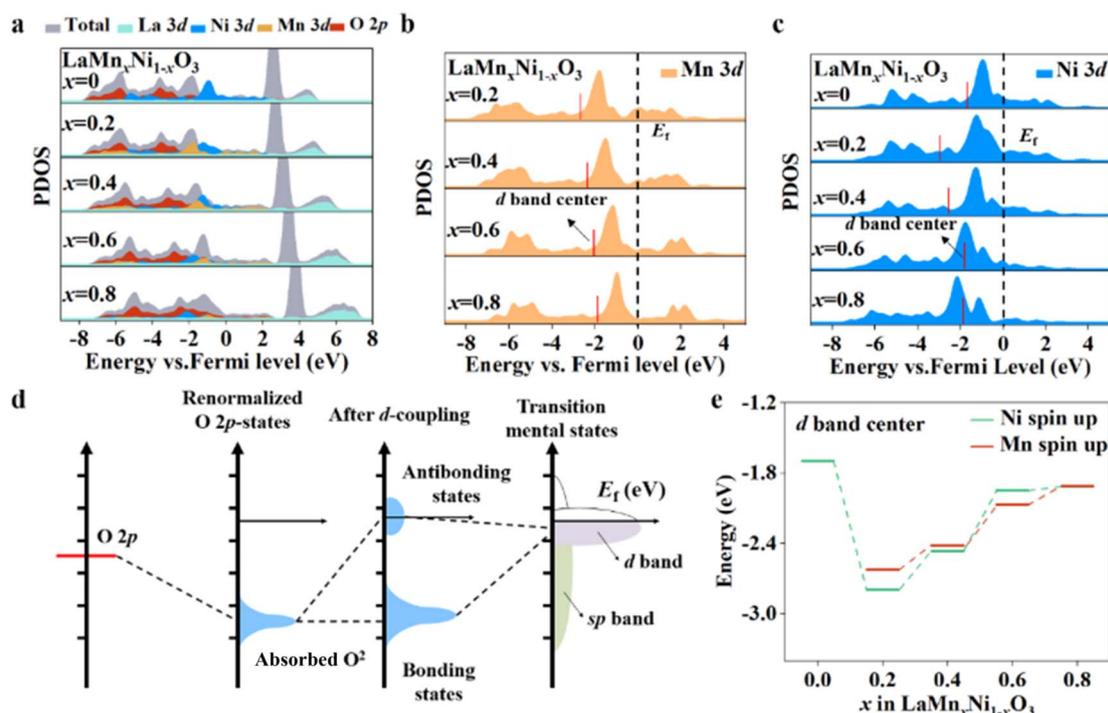
Fig. 6 (a) Comprehensive PDOS for various elements in LaMn<sub>x</sub>Ni<sub>1-x</sub>O<sub>3</sub>. (b) PDOS of Mn 3d orbitals in LaMn<sub>x</sub>Ni<sub>1-x</sub>O<sub>3</sub>. (c) PDOS of Ni 3d orbitals in LaMn<sub>x</sub>Ni<sub>1-x</sub>O<sub>3</sub>. (d) Schematic diagram illustrating the shift of the d band center. (e) Trend analysis of the d band center variations for Mn and Ni.
