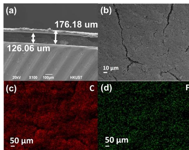
Fig. 4 SEM images of (a) the cross-sectional view of the super P coated separator, (b) the front view of the super P coated separator (500 $\times$ ), (c) and (d) the corresponding elemental mapping.
