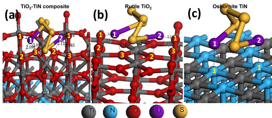
Fig. 8 Optimized geometries illustrating the adsorption of  $\text{Li}_2\text{S}_4$  by (a)  $\text{TiO}_2$ -TiN composite, (b) R- $\text{TiO}_2$  with their corresponding Li-O bond and (c) O-TiN with its Li-N bonds.
