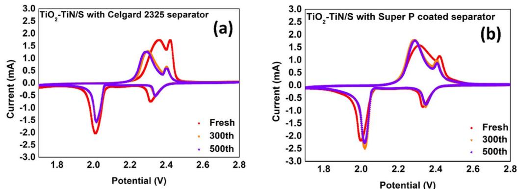
Fig. 9 (a) The CV curves of TiO<sub>2</sub>-TiN/S battery with Celgard 2325 separator, (b) TiO<sub>2</sub>-TiN/S battery with carbon coated separator.
