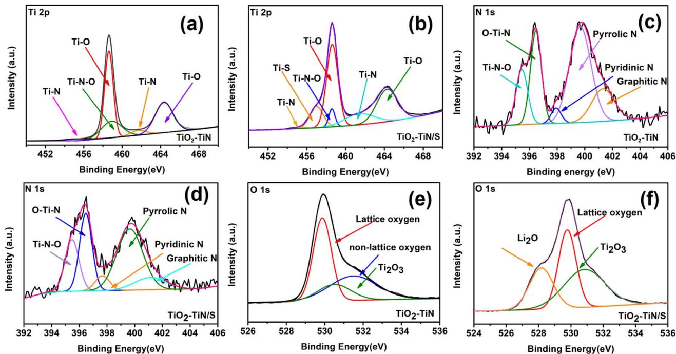
Fig. 5 XPS spectra for (a)  $\text{TiO}_2$ -TiN composite Ti 2p, (b)  $\text{TiO}_2$ -TiN composite/S Ti 2p, (c)  $\text{TiO}_2$ -TiN composite N 1s, (d)  $\text{TiO}_2$ -TiN composite/S N 1s, (e)  $\text{TiO}_2$ -TiN composite O 1s, (f)  $\text{TiO}_2$ -TiN composite/S O 1s.
