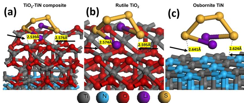
Fig. 7 Optimized geometries illustrating the adsorption of  $\text{Li}_2\text{S}_4$  by (a) the local region of  $\text{TiO}_2$ -TiN composite, (b) R- $\text{TiO}_2$  and (c) O-TiN with their corresponding Ti-S bonds.
