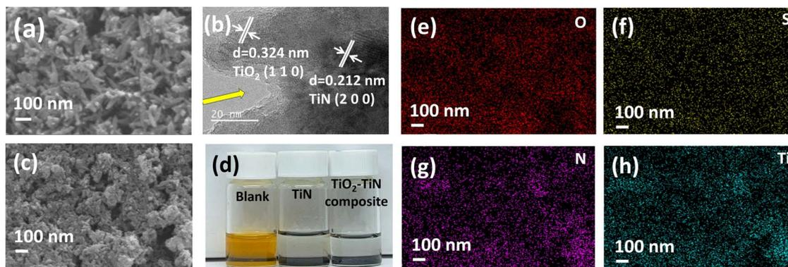
Fig. 3 (a) SEM image, (b) TEM images, (c) SEM images, (d) the visual adsorption experiment of  $\text{TiO}_2$ –TiN composite and (e–h) the corresponding elemental mapping.
