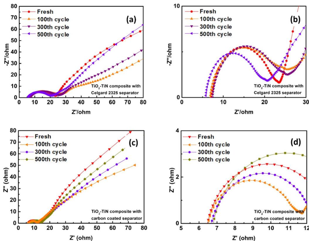
Fig. 10 Nyquist plots of (a and b) TiO<sub>2</sub>-TiN/S battery with Celgard 2325 separator and (c and d) TiO<sub>2</sub>-TiN/S battery with carbon coated separator.
