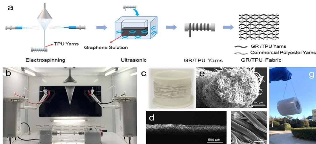
**Fig. 1** (a) Schematic of the fabrication process of the GR/TPU strain sensor. (b) Picture of the nano-yarn instrument. (c) Photographs of TPU yarns. (d–f) SEM images of TPU yarns at different magnifications. (e) Cross-sectional SEM image of the TPU yarns. (g) Photograph of GR/TPU yarns hanging an adhesive tape.
