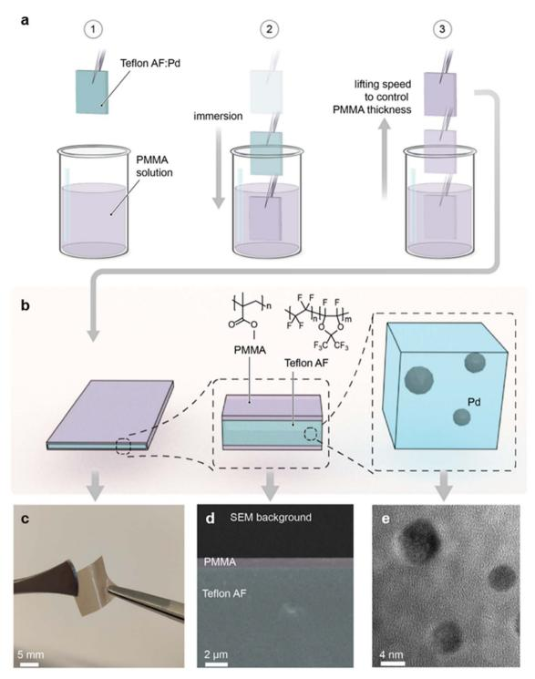
Fig. 2 Preparation and characterization of Teflon AF:Pd – PMMA core:shell structures. (a) Schematic of the dip coating process. (b) Architecture of Teflon AF:Pd films coated with PMMA, including the chemical structures of PMMA and Teflon AF. (c) Photograph of a Teflon AF:Pd film coated with PMMA. (d) False-colored SEM images of the cross section of a Teflon AF:Pd film dip coated with PMMA at 5 mm s<sup>-1</sup>. (e) TEM image of Pd nanoparticles in Teflon AF.
