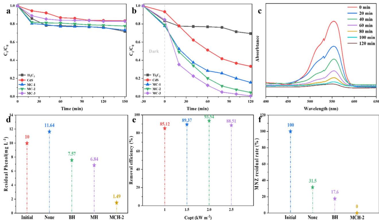
Fig. 6 (a) Static adsorption test of  $\text{Ti}_3\text{C}_2$  MXene/CdS catalysts. (b) Photocatalytic degradation of RhB by  $\text{Ti}_3\text{C}_2$  MXene/CdS samples. (c) UV-vis curves of RhB at different reaction times. (d) Removal of phenol by different hydrogels. (e) Removal rate of phenol by MCH-2 at different light intensities. (f) Purification effect of different hydrogels on metronidazole.
