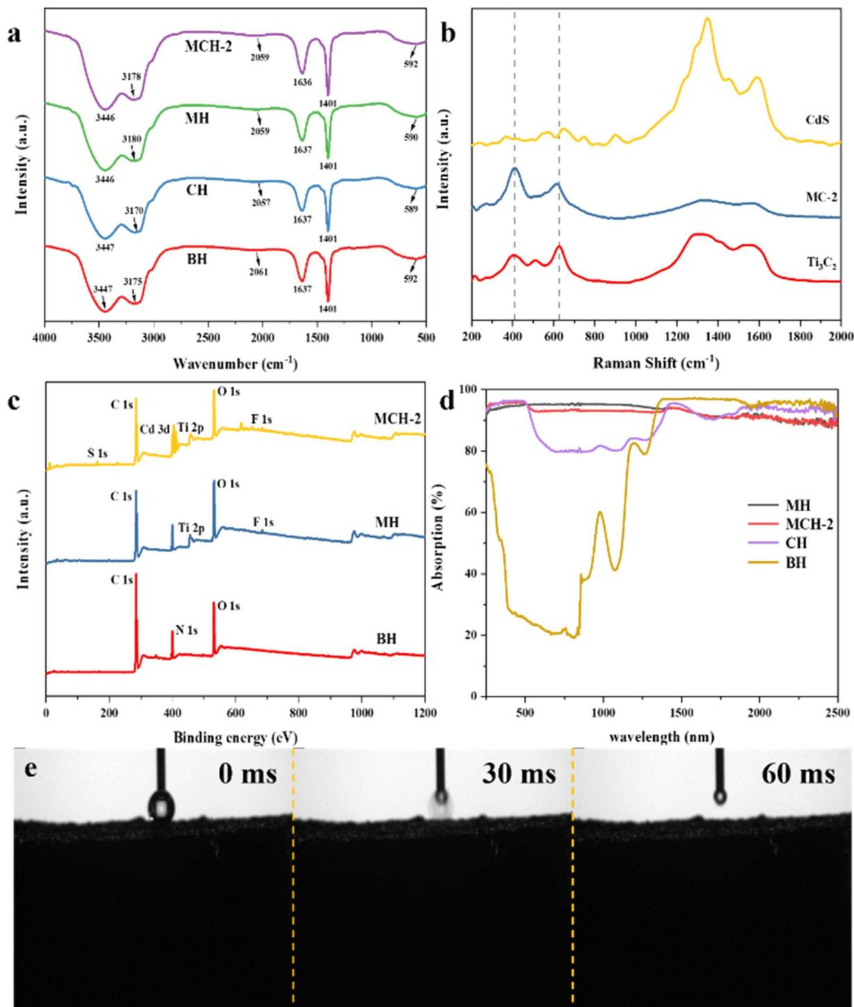
Fig. 4 (a) FTIR spectra of BH, CH, MH, and MCH-2. (b) Raman spectroscopy of Ti<sub>3</sub>C<sub>2</sub>, MC-2, and CdS. (c) XPS spectra of BH, MH, and MCH-2. (d) UV-vis-NIR absorption spectra of hydrogels. (e) Surface contact angle of MCH-2.
