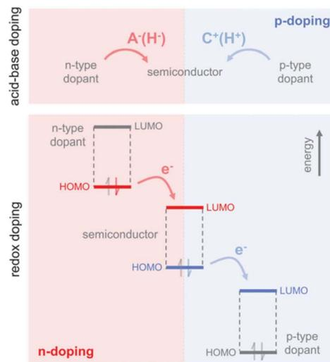
Fig. 3 Mechanisms for n-type and p-type doping: the top panel is acid–base doping showing anion ( $H^-$ ) or cation ( $H^+$ ) addition to the polymer backbone. The bottom panel is redox doping, showing the transfer of electrons to the LUMO level or the transfer of electrons from the HOMO level of the polymer. Reproduced with permission.<sup>143</sup> Copyright, 2017, Wiley – *Advanced Materials*.
