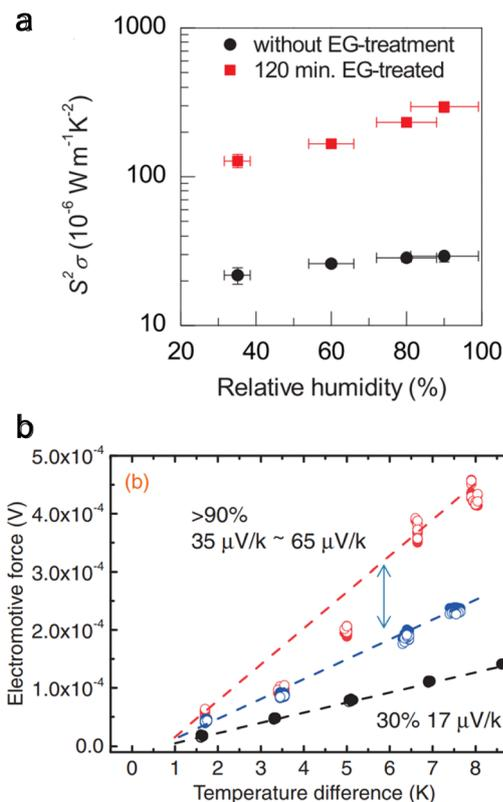
Fig. 25 Effect of relative humidity on thermoelectric properties. (a) The power factor for pristine and 120 min EG-treated PEDOT:PSS films at varying humidity. Reproduced with permission<sup>44</sup> Copyright, 2016 American Physical Society – APL. (b) Thermoelectric voltage for varying temperatures and different humidity variations. Reproduced with permissions.<sup>333</sup> Copyright, 2014, The Japan Society of Applied Physics – APE.
