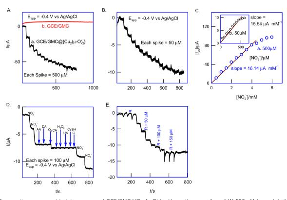
Fig. 12 Comparative amperometric i-t responses of GCE/GMC@ $\{Cu_2(\mu-O)_2\}$  with continuous spikes of (A) 500  $\mu$ M (curve b is the control response of the GCE/GMC) and (B) 50  $\mu$ M NO $_2^-$ ; (C) calibration plots of  $i_{pc}$  vs. [NO $_2^-$ ] in different NO $_2^-$  concentration regions. (D) Effect of interference of various analytes. (E) Analysis of a tap water sample.
