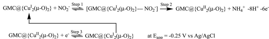
**Scheme 2** Reaction mechanism on the GMC@{Cu<sub>2</sub>(μ-O)<sub>2</sub>} for the electrocatalytic reduction of nitrite to ammonium under electrochemical (step 3) and chemical (steps 1 & 2) conditions. [GMC@{Cu<sub>2</sub>(μ-O)<sub>2</sub>}⋯NO<sub>2</sub><sup>-</sup>] is an intermediate species similar to Scheme 1D.
