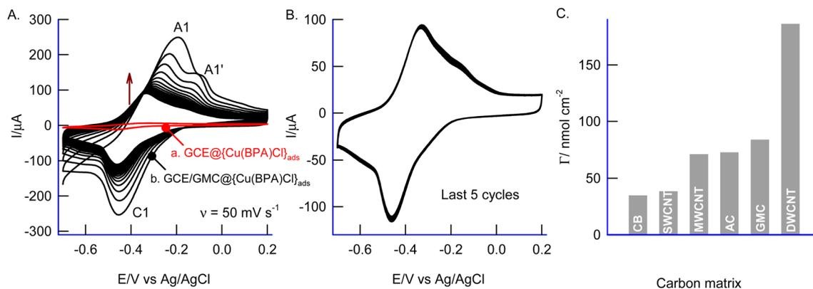
Fig. 1 (A) Cyclic voltammograms of (a)  $\text{GCE}@{\text{Cu}(\text{BPA})\text{Cl}}_{\text{ads}}$ ; (b)  $\text{GCE}/\text{GMC}@{\text{Cu}(\text{BPA})\text{Cl}}_{\text{ads}}$  in nitrogen-purged 0.1 M PBS, pH 7, at scan rate ( $\nu$ ) = 50  $\text{mV s}^{-1}$  ( $n = 20$  cycles) and (B) last five CVs; (C) comparative plots of surface excess values of different carbon nanomaterials used.
