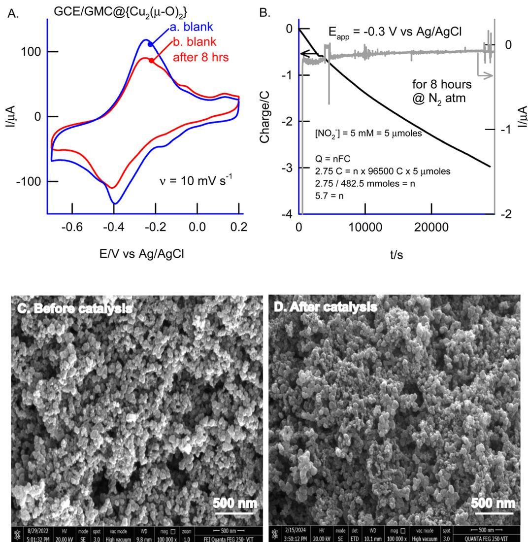
**Fig. 10** (A) CV responses of GCE/GMC@{Cu<sub>2</sub>(μ-O)<sub>2</sub>} before and after the bulk electrolysis of 5 mM NO<sub>2</sub><sup>-</sup> at an applied potential of -0.3 V vs. Ag/AgCl in N<sub>2</sub> purged pH 2 HCl-KCl. (B) Bulk electrolysis response (inset: number of electrons calculation). Comparison of GCE/GMC@{Cu<sub>2</sub>(μ-O)<sub>2</sub>} before (C) and after (D) electrocatalytic nitrite reduction.
