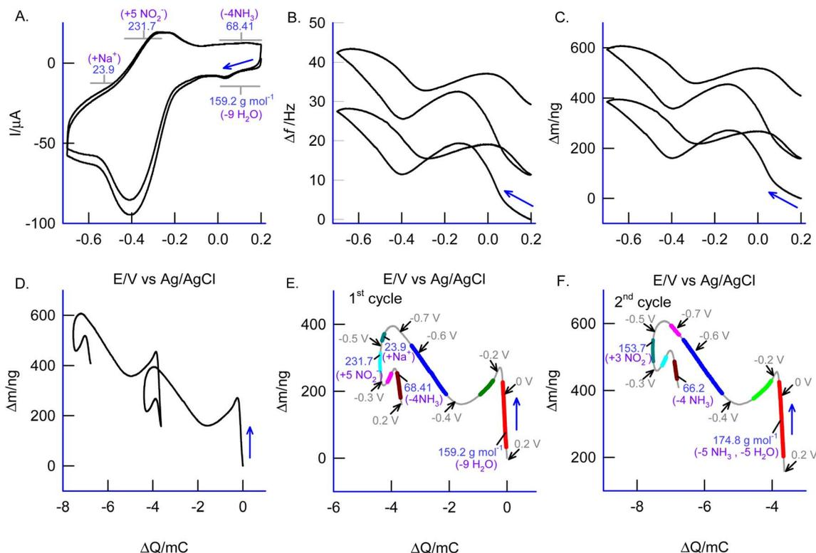
Fig. 9 (A and B) *In situ* CV-EQCM responses of GCE/GMC@ $\{\text{Cu}_2(\mu\text{-O})_2\}$  with  $500 \mu\text{M NO}_2^-$  in  $\text{N}_2$  purged pH 7 PBS at a scan rate of  $10 \text{ mV s}^{-1}$ . Corresponding derivative plots of (C)  $\Delta m$  vs.  $E$  and  $\Delta m$  vs.  $\Delta Q$  of (D) 1–2 cycles, (E) the first cycle and (F) second cycle.
