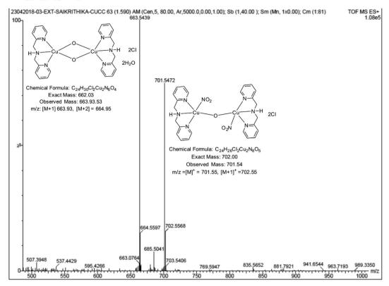
Fig. 11 ESI-MS data of an ethanolic extract of GCE/GMC@ $\{Cu_2(\mu-O)_2\}$ , upon  $NO_2^-$  electrocatalysis.
