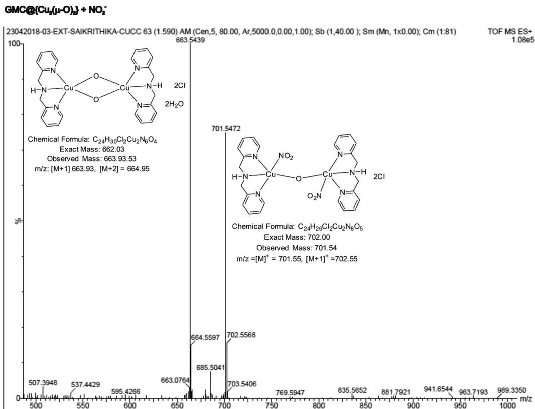
Fig. 11 ESI-MS data of an ethanolic extract of GCE/GMC@{Cu<sub>2</sub>(μ-O)<sub>2</sub>}, upon NO<sub>2</sub><sup>-</sup> electrocatalysis.
