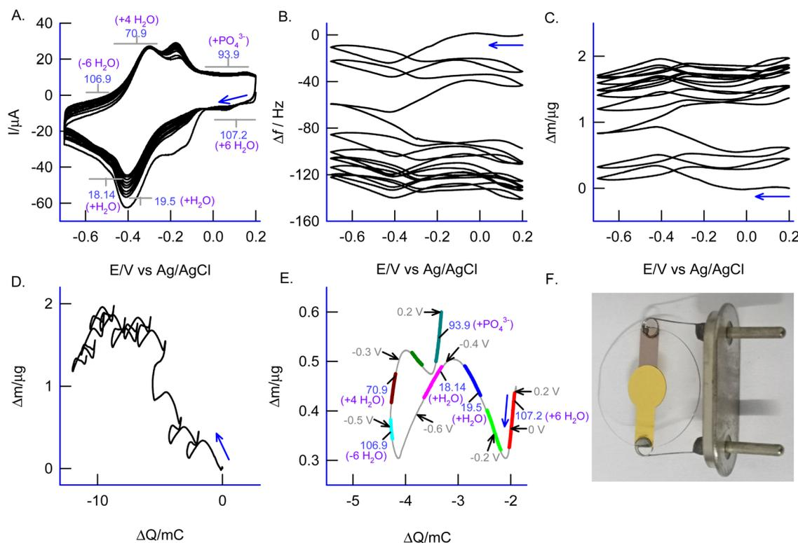
Fig. 5 (A and B) *In situ* CV-EQCM responses of  $\text{GCE}/\text{GMC}@{\text{Cu}(\text{BPA})\text{Cl}}_{\text{ads}}$  in  $\text{N}_2$  purged 0.1 M PBS, pH 7, at a scan rate of  $10\text{ mV s}^{-1}$ . Inset of (A) shows the molecules involved in the redox reaction. Corresponding derivative plots of (C)  $\Delta m$  vs.  $E$  and  $\Delta m$  vs.  $\Delta Q$  plots of (D) 1–10 cycles and (E) second cycle. (F) Picture of an EQCM-Au electrode.
