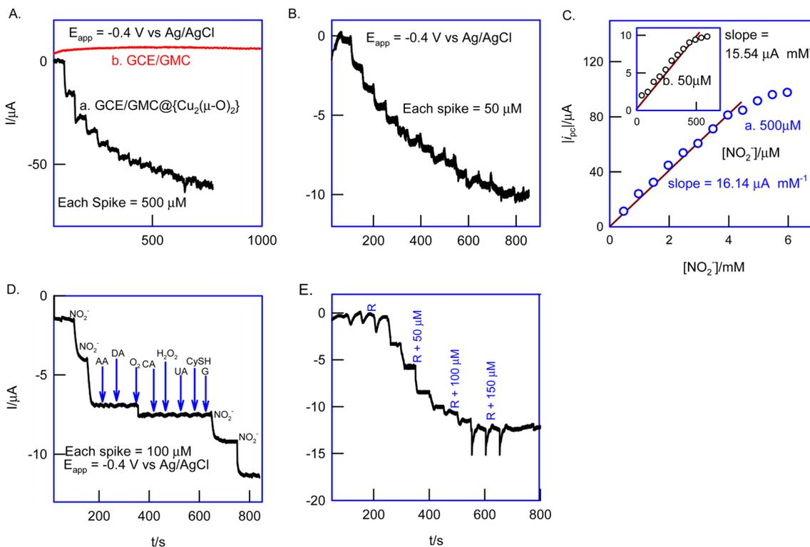
Fig. 12 Comparative amperometric  $i-t$  responses of GCE/GMC@{Cu<sub>2</sub>(μ-O)<sub>2</sub>} with continuous spikes of (A) 500 μM (curve b is the control response of the GCE/GMC) and (B) 50 μM NO<sub>2</sub><sup>-</sup>; (C) calibration plots of  $i_{pc}$  vs. [NO<sub>2</sub><sup>-</sup>] in different NO<sub>2</sub><sup>-</sup> concentration regions. (D) Effect of interference of various analytes. (E) Analysis of a tap water sample.
