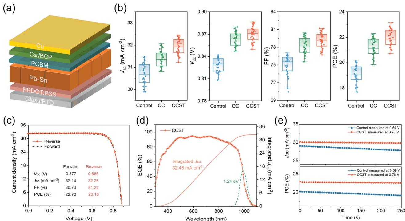
Fig. 4 (a) Device architecture of Sn–Pb PSCs. (b) Statistics of the photovoltaics parameters of the control, CC, and CCST PSCs. (c)  $J$ - $V$  curves of the champion CCST device. (d) EQE spectra and the integrated  $J_{sc}$  of the CCST device; (e) steady-state photocurrent and PCE output at the maximum power point.
