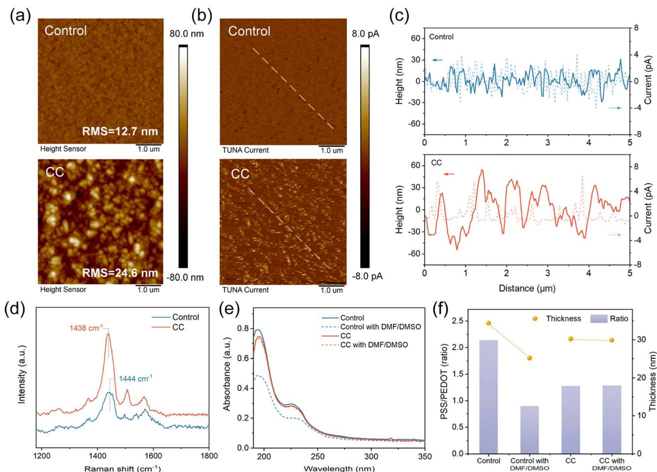
**Fig. 1** (a) AFM morphology, (b) tunneling AFM current mapping, and (c) height/current along scan distance of the PEDOT:PSS films without (control) and with CC; the scan is along a line shown in the picture of (b). (d) Raman spectra of the PEDOT:PSS films without (control) and with CC. (e) UV absorption spectra of the PEDOT:PSS films without and with DMF/DMSO treatment. (f) Layer thickness and PSS/PEDOT molar ratio of the PEDOT:PSS films without and with DMF/DMSO treatment.
