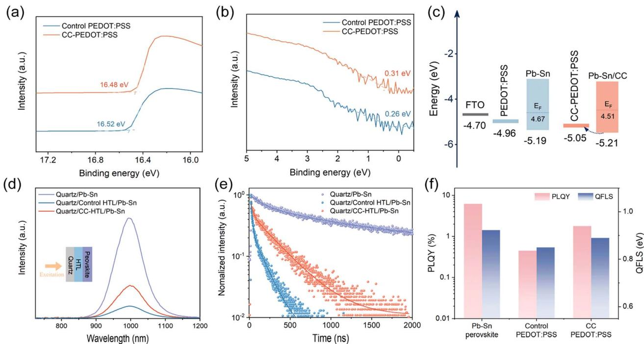
Fig. 3 UPS spectra of the control and CC-PEDOT:PSS films, (a) cut-off region and (b) valence band edge region. (c) Energy level diagram of the FTO/HTL/perovskite half stack. (d) PL spectra, (e) time-resolved PL spectra, and (f) PLQY and QFLS values for neat perovskite film, perovskite/control HTL, and perovskite/CC-HTL.
