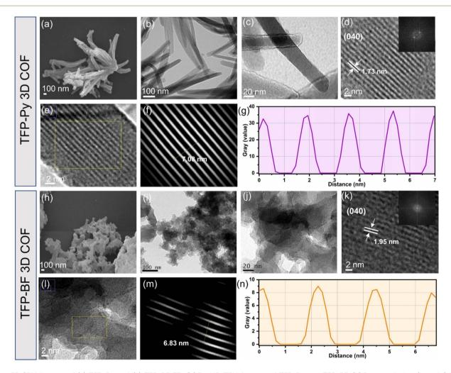
Fig. 4 FE-SEM images of (a) TFP-Py and (h) TFP-BF 3D COFs. HR-TEM images of TFP-Py and TFP-BF COFs recorded at (b and i) highmagnification, with a scale bar of 100 nm, and (c-e, j-l) low-magnification, with (c - and j) a scale bar of 20 nm and (d, e, k) and (inset: the SAED pattern. The FFT image from the corresponding yellow square using the image J software of (f) TFP-Py and (m) TFP-BF 3D COFs. The simulated FFT diagrams of a yellow selected square of (g) TFP-Py and (n) TFP-BF 3D COFs.
