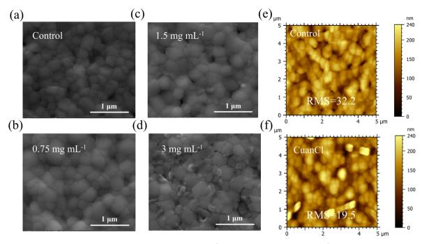
Fig. 4 SEM images of the perovskite films: (a) control, (b)  $0.75 \text{ mg mL}^{-1}$  CuanCl-treated, (c)  $1.5 \text{ mg mL}^{-1}$  CuanCl-treated and (d)  $3 \text{ mg mL}^{-1}$  CuanCl-treated. AFM images of perovskite films: (e) control and (f) CuanCl treated.
