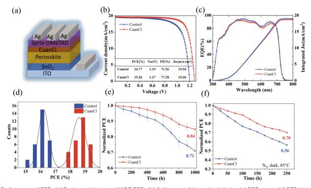
Fig. 6 Performance of PSCs. (a) Device architecture of WBG PSCs. (b) J-V curves of the optimal device. (c) EQE curves. (d) PCE histogram of WBG PSCs prepared with and without CuanCl treatment. (e) Long-term stability of the two devices under non-encapsulated conditions with a relative humidity of  $40\% \pm 10\%$ . (f) The change in PCE for unencapsulated devices under exposure to an 85 °C  $N_2$  atmosphere.
