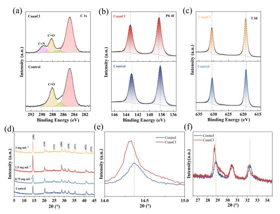
Fig. 2 XPS spectra of (a) C 1s, (b) Pb 4f, and (c) | 3d. (d) XRD patterns. (e) The zoomed-in view of the (100) peak. (f) Amplification of (200) and (210) peaks.
