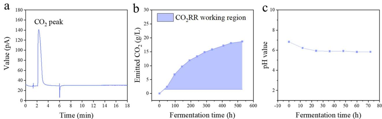
Fig. 2 Fermentation emissions and broth condition. (a) Gas chromatography of fermentation-emitted  $\text{CO}_2$ .  $\text{CO}_2$  is the only gas product. (b) Amount of fermentation-emitted  $\text{CO}_2$  and (c) pH value of the fermentation broth over time.
