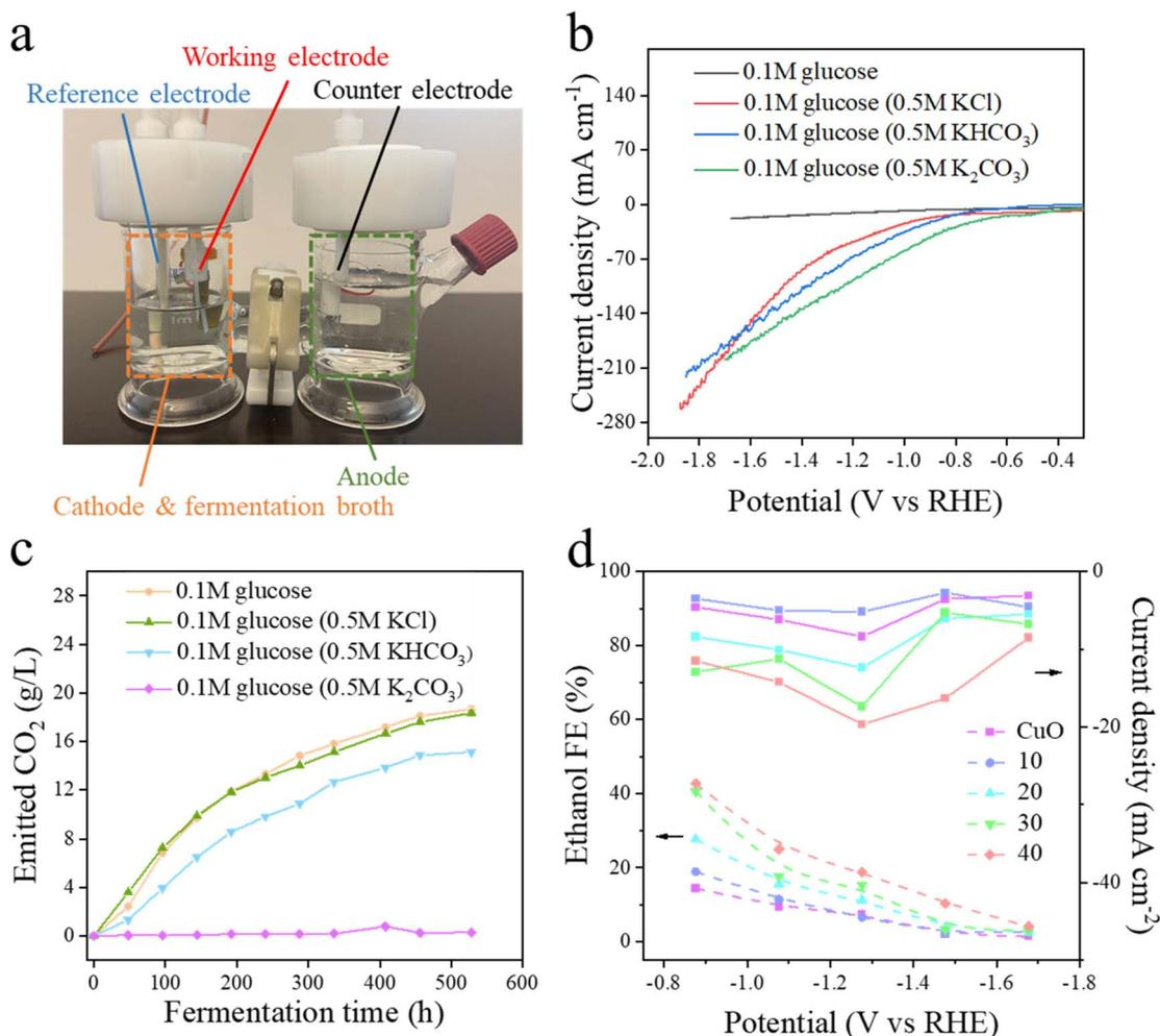
Fig. 4 CO<sub>2</sub>RR performance in the fermentation–CO<sub>2</sub>RR hybrid cell. (a) Photo of the fermentation–CO<sub>2</sub>RR hybrid cell. (b) LSV curves of the CuO–Ag catalyst in different solutions. (c) Amount of fermentation CO<sub>2</sub> emissions in various glucose solutions. (d) Ethanol FEs and partial current densities with different CuO–Ag interface numbers (0, 10, 20, 30, and 40) in 0.1 M glucose (0.5 M KCl).
