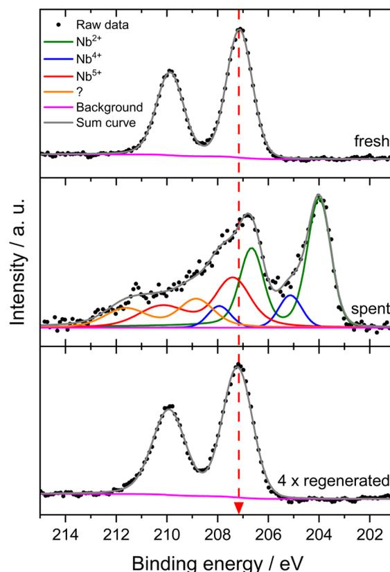
**Fig. 7** Intensity-normalized XP spectra for the Nb 3d level of the 6Mo1Nb/HZSM-5 catalyst before the reaction (bottom), after the reaction with methane at 700 °C for 360 min (middle) and after four reaction/regeneration cycles. Reaction conditions: 700 °C, 300 mg catalyst, 90% CH<sub>4</sub> + 10% N<sub>2</sub>, 3200 SCC g<sub>cat</sub><sup>-1</sup> h<sup>-1</sup>, 1 atm, 6 h. Regeneration: 450 °C, air, 1100 SCC g<sub>cat</sub><sup>-1</sup> h<sup>-1</sup>, 1 atm, 45 min.
