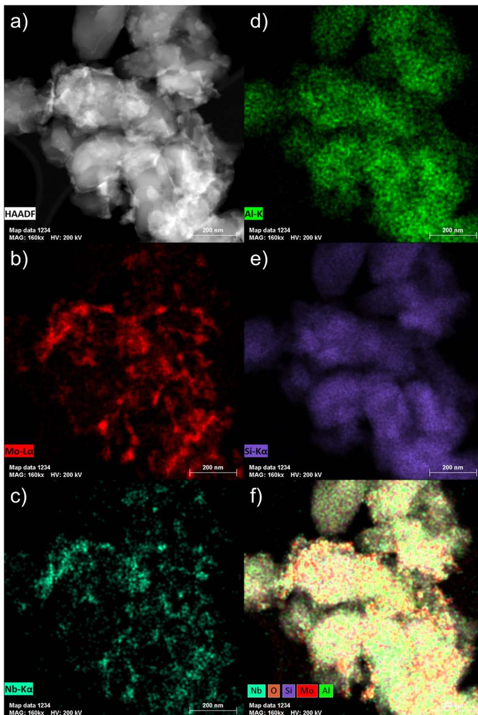
Fig. 5 STEM micrograph (a) and the corresponding EDS maps ((b) Mo  $L\alpha$ ; (c) Nb  $K\alpha$ ; (d) Al  $K$ ; (e) Si  $K\alpha$ ; (f) overlay of O, Si, Al, Mo and Nb) of the fresh 6Mo1Nb/HZSM-5 catalyst.
