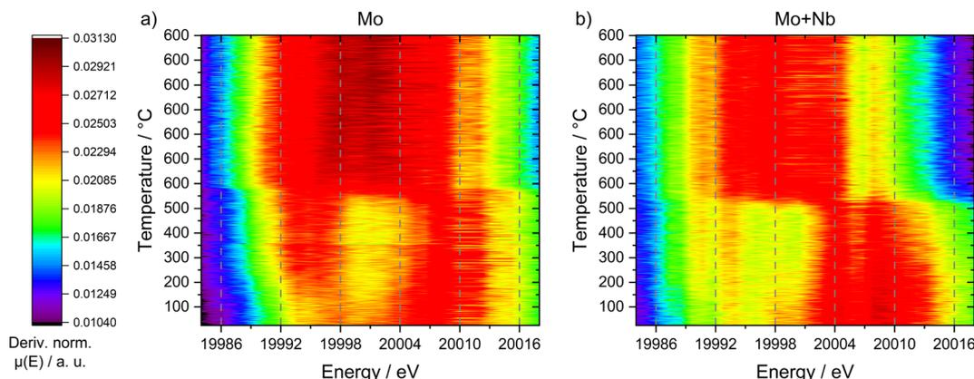
Fig. 10 Heatmap depictions of the first derivative of all recorded XANES measurements during the temperature-programmed reaction of 6Mo/HZSM-5 (a) and 6Mo1Nb/HZSM-5 (b) with 50 mL min<sup>-1</sup> 20% CH<sub>4</sub>/N<sub>2</sub> at 1 atm and a heating rate of 10 °C min<sup>-1</sup>.
