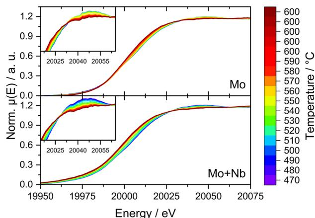
Fig. 9 Normalized XANES at the Mo K-edge recorded *in situ* of 6Mo/HZSM-5 (top) and 6Mo1Nb/HZSM-5 (bottom) during continuous heating. Curves depict the normalized sum of 10 measurements (60 s) in the range of  $T \pm 5$  °C. Insets show zoom-ins on the edge features. Reaction conditions: 50 mL min<sup>-1</sup> 20% CH<sub>4</sub>/N<sub>2</sub>, 1 atm, heating rate 10 °C min<sup>-1</sup>, heating from RT to 600 °C.
