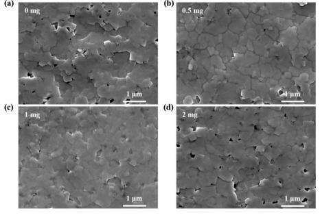
Fig. 2 Representative SEM images of PEA<sub>0.2</sub>FA<sub>0.8</sub>SnI<sub>3</sub> films with (a) 0 mg, (b) 0.5 mg, (c) 1 mg and (d) 2 mg 2-aminopyrimidine.
