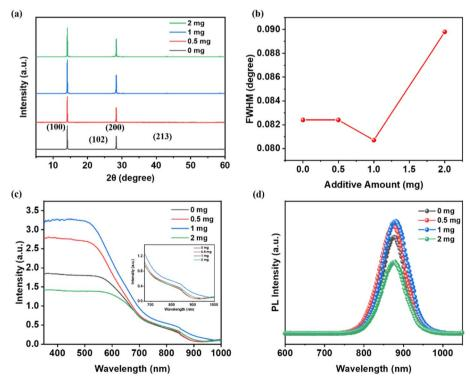
Fig. 1 (a) XRD diffraction patterns and (b) the FWHM of the (100) peak for  $PEA_{0.2}FA_{0.8}SnI_3$  films with varying amounts of 2-aminopyrimidine (0– 2 mg). (c) Absorption spectra (the inset shows the enlarged absorption edge) and (d) PL spectra of PEA<sub>0.2</sub>FA<sub>0.8</sub>SnI<sub>3</sub> films with varying amounts of 2-aminopyrimidine.
