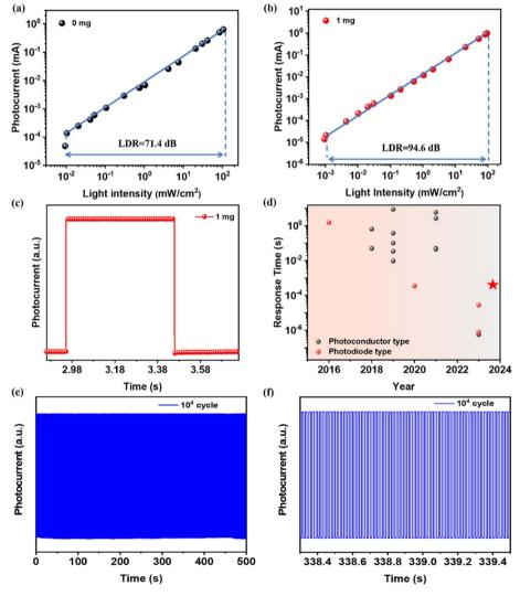
Fig. 5 (a and b) Photocurrent as a function of incident light intensity. (c) Response time of the  $PEA_{0.2}FA_{0.8}SnI_3$ -based PD with 1 mg 2-aminopyrimidine. (d) Response times of previously reported  $PEA_{0.2}FA_{0.8}SnI_3$ -based PDs. (e) Long-term I-t curve for the  $PEA_{0.2}FA_{0.8}SnI_3$ -based PD with 1 mg 2-aminopyrimidine under 533 nm green light illumination. (f) Enlarged I-t curve.
