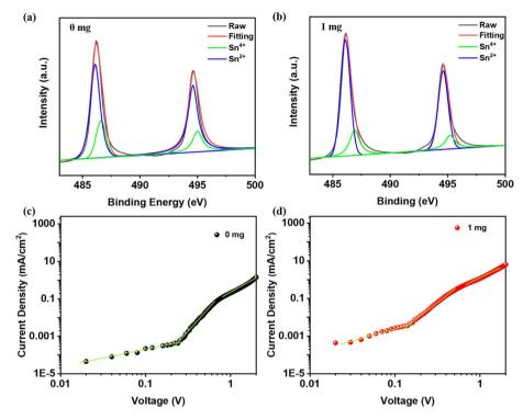
Fig. 3 (a and b) XPS spectra, and (c and d) J-V curves for the electron-only devices based on the PEA<sub>0.2</sub>FA<sub>0.8</sub>SnI<sub>3</sub> films without and with 1 mg 2-aminopyrimidine.
