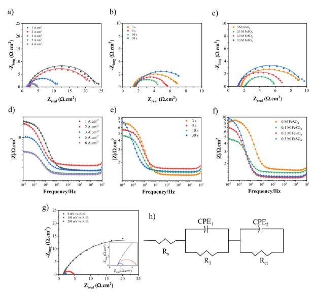
Fig. 10 The Nyquist curves and Bode plots at an overpotential of -100 mV for electrodes fabricated at different (a and d) electrodeposition current densities, (b and e) duration times, and (c and f) FeSO<sub>4</sub> concentrations, (g) Nyquist curves of Ni-Fe-S 5 A cm<sup>-2</sup>/10 s/0.1 M at different overpotentials, and (h) equivalent circuit.
