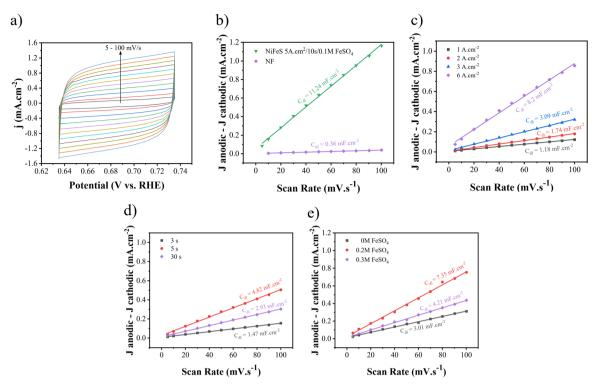
Fig. 9 (a) CV curves with different scan rates (5–100 mV s<sup>-1</sup>) and  $C_{dl}$  plots for (b) optimum Ni–Fe–S and NF and Ni–Fe–S synthesized at (c) different electrodeposition current densities, (d) different duration times, and (e) different concentrations of FeSO<sub>4</sub>.
