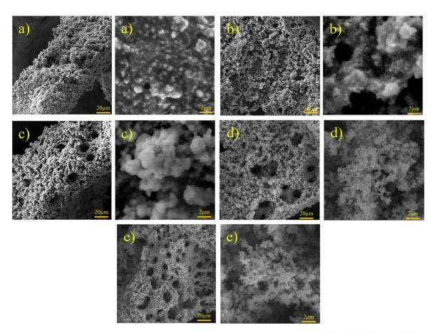
Fig. 2 FESEM images of Ni–Fe–S with magnifications of  $1k\times$  and  $10k\times$  at 10 s, 0.1 M FeSO<sub>4</sub>, and (a) 1, (b) 2, (c) 3, (d) 5, and (e) 6 A cm<sup>-2</sup>.
