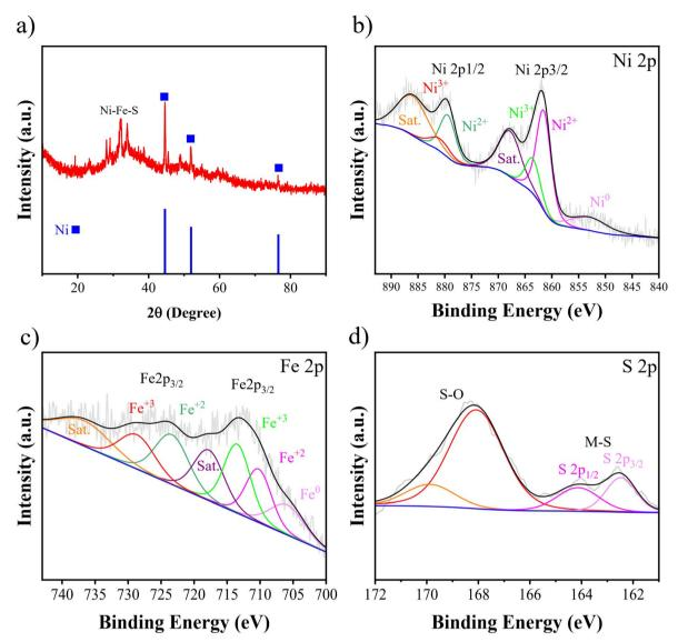
(a) XRD pattern and high resolution XPS spectra of (b) Ni, (c) Fe, and (d) S for optimum Ni-Fe-S 5 A cm<sup>-2</sup>/10 s/0.1 M.
