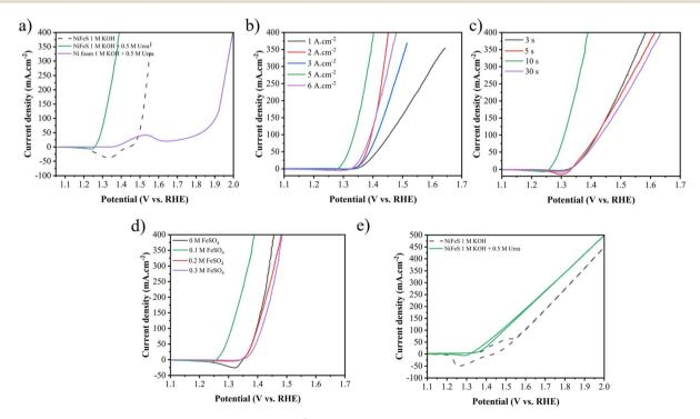
Fig. 8 (a) LSV curves of NF for the UOR and Ni-Fe-S 5 A cm<sup>-2</sup>/10 s/0.1 M for the UOR and OER, LSV curves of the synthesized electrodes with different (b) applied current densities, (c) duration times, and (d)  $FeSO_4$  concentrations in 1 M KOH + 0.5 M urea electrolyte, and (e) LSV curves of 2 electrode system Ni-Fe-S 5 A cm<sup>-2</sup>/10 s/0.1 M||Ni-Fe-S 5 A cm<sup>-2</sup>/10 s/0.1 M towards overall urea oxidation and water splitting
