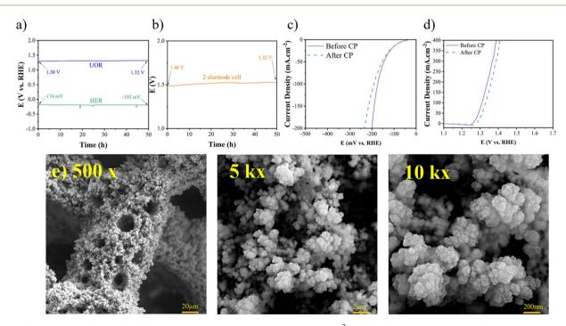
Fig. 12 (a) CP for the HER, UOR, and (b) 2 electrode system recorded at 100 mA cm<sup>-2</sup> for 50 h, LSV curves after CP for (c) HER and (d) UOR, and (e) FESEM images after CP with different magnifications of 500×, 1k×, and 10k×.
