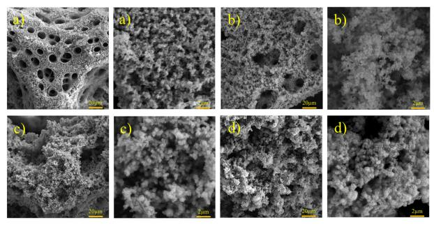
Fig. 4 FESEM images of Ni-Fe-S with magnifications of 1k× and 10k× at 5 A cm<sup>-2</sup>, 10 s, and (a) 0, (b) 0.1, (c) 0.2, and (d) 0.3 M FeSO<sub>4</sub>.
