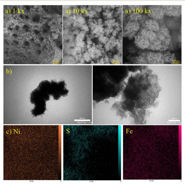
Fig. 5 (a) FESEM images with magnifications of  $1k \times$ ,  $10k \times$ , and  $100k \times$ , (b) TEM images and (c) elemental mapping with magnification of  $5k \times$  for optimum Ni–Fe–S 5 A cm<sup>-2</sup>/10 s/0.1 M.
