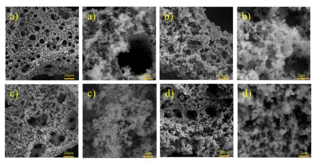
Fig. 3 FESEM images of Ni-Fe-S with magnifications of  $1k\times$  and  $10k\times$  at 5 A cm<sup>-2</sup>, 0.1 M FeSO<sub>4</sub>, and (a) 3, (b) 5, (c) 10, and (d) 30 s.
