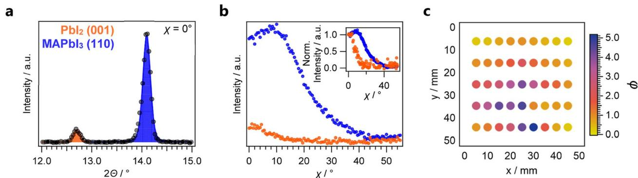
Fig. 2 XRD characterization of the combinatorial MAPbI<sub>3</sub> sample. (a) 2-Theta scan for a selected sample and (b) Azimuthal  $\chi$ -scan for the same sample. The inset depicts traces that have been normalized at  $\chi = 0^\circ$ , according to the term defined in eqn (3). Based on these individual results, the conversion ratio is calculated for each sample. (c) Conversion ratio  $\phi$  as function of the position on the combinatorial library.
