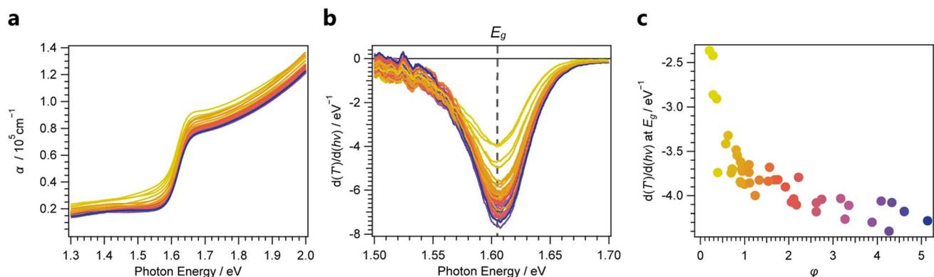
Fig. 3 (a) Absorption coefficients  $\alpha$  with varying  $\phi$ . (b) First derivative of the reflection-corrected transmission  $T'$ , showing the steepness of the transmission onset near the bandgap  $E_g$ . (c) Extracted values of subplot b, indicating a clear correlation between the MHP/PbI<sub>2</sub> and the steepness of the transmission onset near the bandgap.
