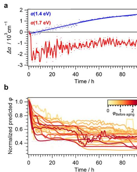
Fig. 6 (a) Observation of the change in optical absorption  $\Delta\alpha$  for a representative sample with  $\phi_{\text{Before aging}} = 0.90$  and thus large amounts of scattering effects as evident from the absorption increase below the bandgap. (b) Normalized predicted kinetic traces expressed as changes in  $\phi$  for samples with low MAPbI<sub>3</sub> phase ratios ( $\phi < 2.5$ ), showing a continuous decrease.
