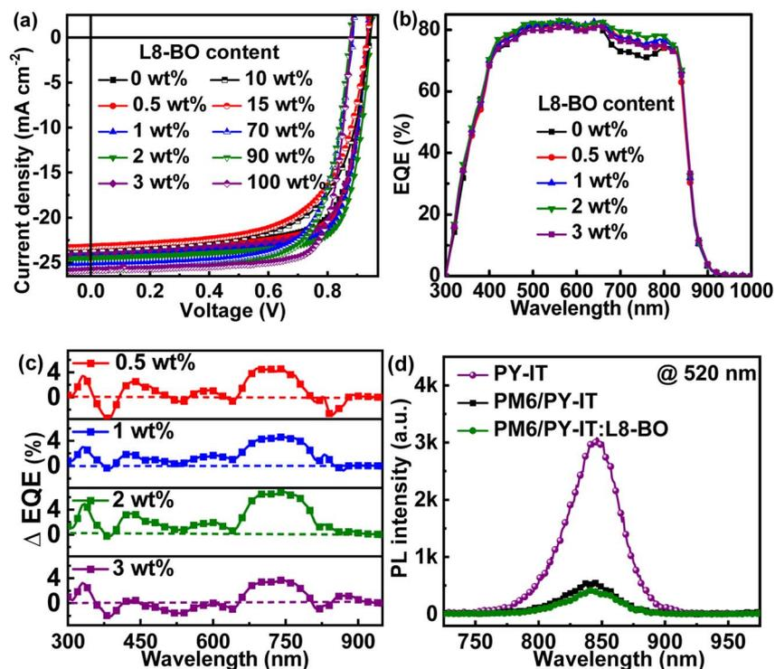
Fig. 2 (a) The  $J$ - $V$  curves of QLA-PSCs with different L8-BO content in the PY-IT layer. (b) The EQE spectra of QLA-PSCs with L8-BO as a solid additive in the PY-IT layer. (c)  $\Delta$ EQE between corresponding QLA-PSCs. (d) PL spectra of neat PY-IT, PM6/PY-IT and PM6/PY-IT:L8-BO films.
