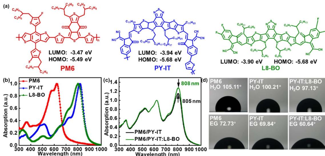
Fig. 1 (a) Chemical structures and energy level of PM6, PY-IT and L8-BO. (b) The normalized absorption spectra of PM6, PY-IT and L8-BO. (c) The absorption spectra of PM6/PY-IT and PM6/PY-IT:L8-BO films normalized according to the absorption intensity of PM6. (d) Images of contact angles of PM6, PY-IT and PY-IT:L8-BO films.
