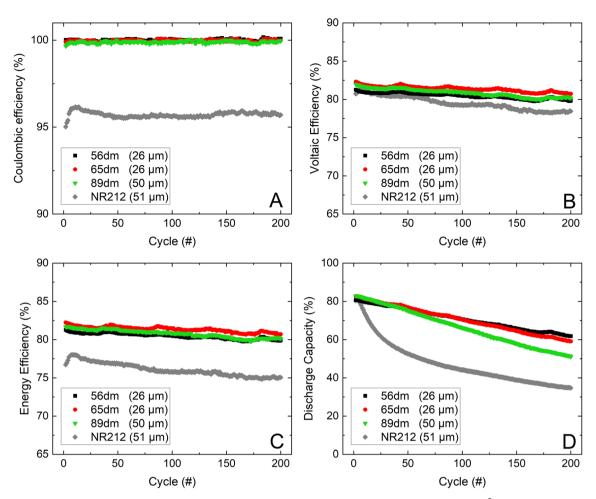
Fig. 8 The cycling performance of the HMT-PMBI variants and Nafion™ NR212 over 200 cycles at 200 mA cm<sup>-2</sup>, with the coulombic efficiency (A), voltaic efficiency (B), energy efficiency (C) and normalized discharge capacity (D).
