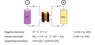
Fig. 1 Schematic depiction of a vanadium redox flow battery in its charged state.
