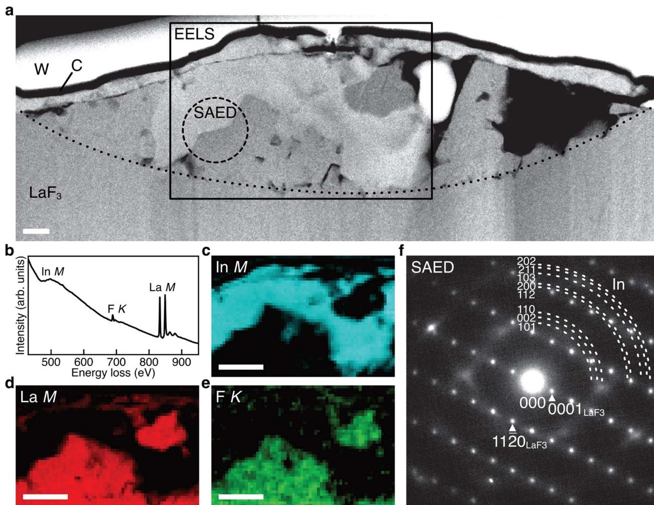
Fig. 4 STEM data obtained from the (In + LaF<sub>3</sub>) anode after one cycle. (a) ADF STEM image obtained from the anode of a battery after one cycle. (b–e) EELS spectrum and In M-, La M-, and F K-edge intensity maps obtained from the rectangle region in (a). (f) SAED pattern obtained from the dashed circle region in (a). The scale bar in (a) is 200 nm and the scale bars in (c)–(e) are 500 nm.
