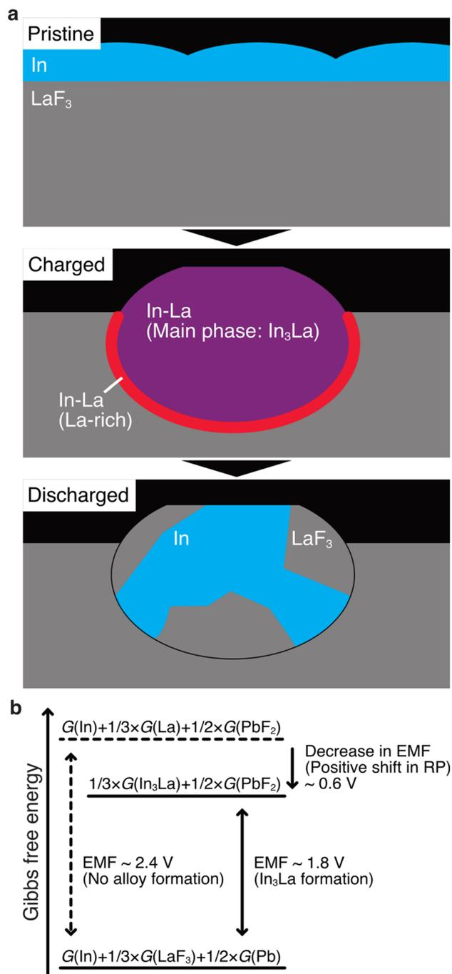
Fig. 5 Schematics for the discussion on the potential shift. (a) The microstructure evolution of the (In + LaF<sub>3</sub>) composite anode. (b) Magnitudes of the Gibbs free energies for the discharged state, charged state with no alloy formation, and charged state with In<sub>3</sub>La formation.
