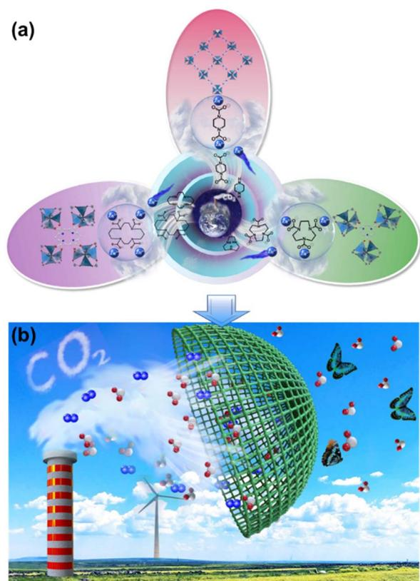
Fig. 1 Schematic diagram of synthetic MOFs and membrane separation. (a) Schematic diagram of the process for MOF synthesis from Zn clusters and various nitrogen-rich heterocycles by introducing CO<sub>2</sub> at room temperature and atmospheric pressure via a one-pot method. (b) Membrane separation diagram for CO<sub>2</sub>/N<sub>2</sub> separation.
