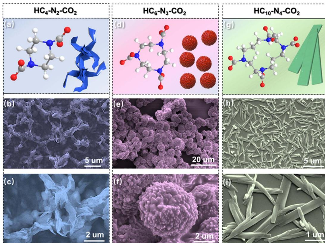
Fig. 2 Molecular structure and morphology of  $\text{HC}_x\text{-N}_y\text{-CO}_2$ : (a–c)  $\text{HC}_4\text{-N}_2\text{-CO}_2$ , (d–f)  $\text{HC}_6\text{-N}_3\text{-CO}_2$ , and (g–i)  $\text{HC}_{10}\text{-N}_4\text{-CO}_2$ . All the ball and stick model states of  $\text{HC}_x\text{-N}_y\text{-CO}_2$  are in the lowest energy states optimized through Chemdraw 3D. Different colored spheres represent different atoms, where blue is N, gray is C, and red is O.
