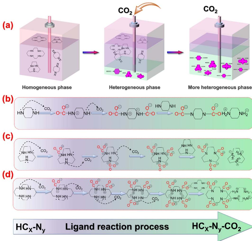
Fig. 3 Formation mechanism of  $\text{HC}_x\text{-N}_y\text{-CO}_2$ . (a) Model process diagram to form  $\text{HC}_x\text{-N}_y\text{-CO}_2$  including mainly three stages (homogeneous phase, heterogeneous phase, and more heterogeneous phase). Mechanisms of ligand formation for MOFs between electrophilic  $\text{CO}_2$  and nucleophilic starting materials. (b)  $\text{HC}_4\text{-N}_2$ . (c)  $\text{HC}_6\text{-N}_3$ . (d)  $\text{HC}_{10}\text{-N}_4$ .
