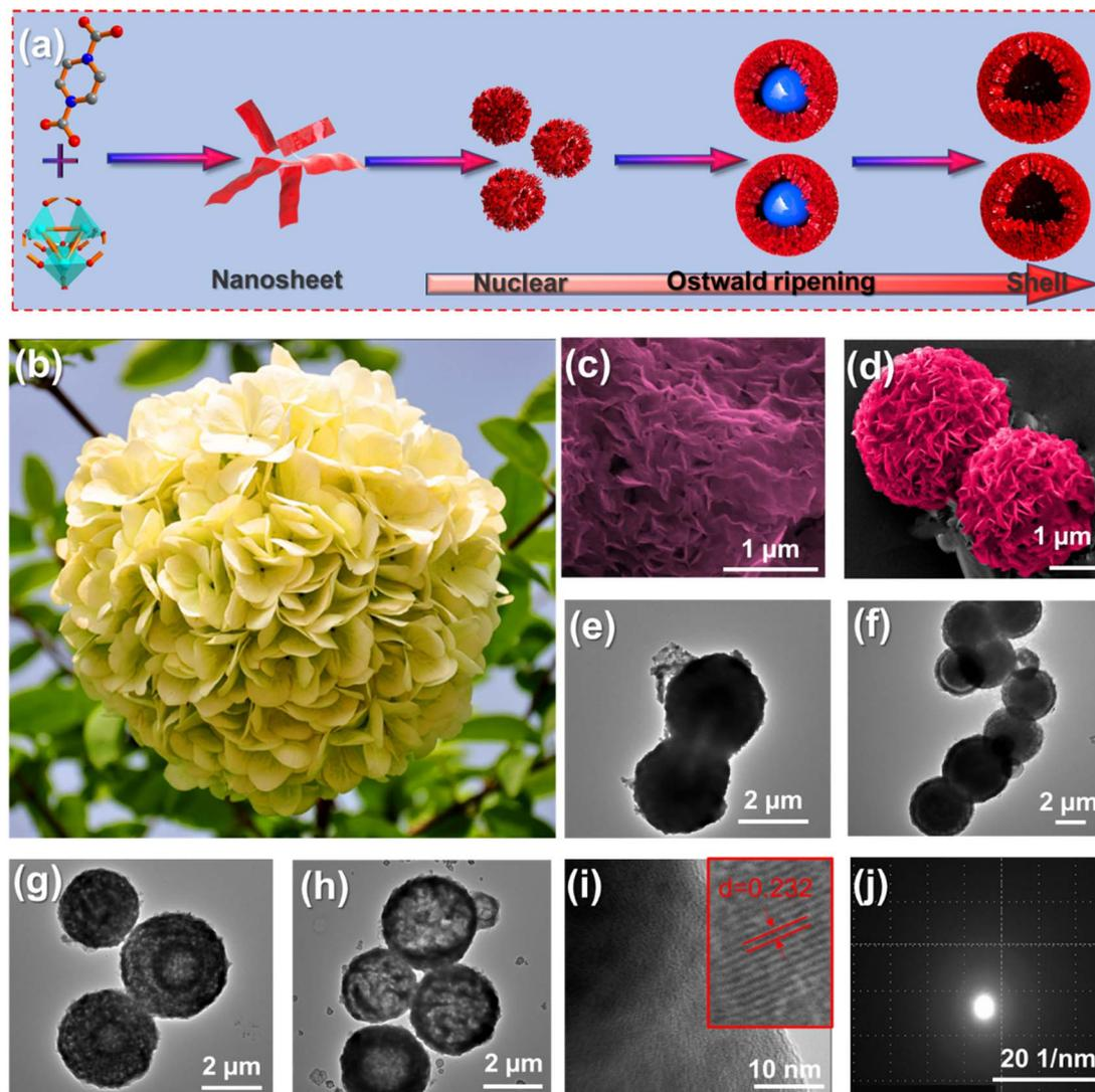
Fig. 4 Formation process of hollow flower-like  $\text{HC}_4\text{-N}_2\text{-CO}_2\text{-ZnSO}_4$ . (a) Model diagram of hollow flower formation according to an inside-out Ostwald ripening process. (b) A digital picture of hydrangea. (c and d) FESEM images. FESEM images were colored red for visual effect. (e–h) Low-magnification TEM images. (i) HR-FETEM image. (j) SAED pattern of  $\text{HC}_4\text{-N}_2\text{-CO}_2\text{-ZnSO}_4$ .
