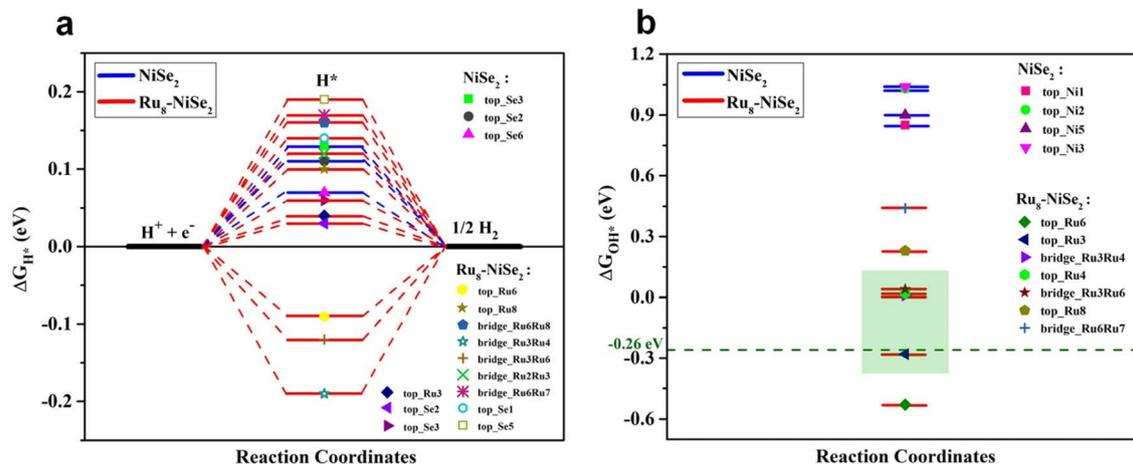
Fig. 6 Theoretical calculations for the HER. (a) Free energy plots for H adsorption and (b) OH adsorption on some of the high symmetry sites of pristine and Ru<sub>8</sub>-NiSe<sub>2</sub> (210) surfaces.
