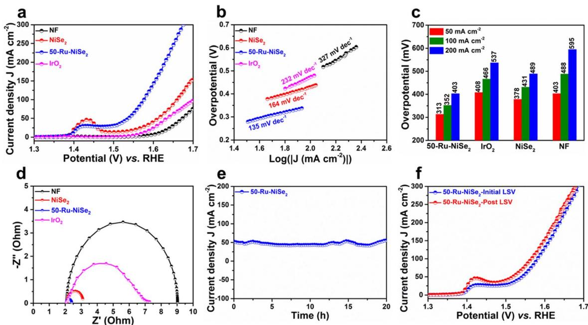
Fig. 4 OER studies. (a) LSV polarization curves of NF, NiSe<sub>2</sub>, 50-Ru-NiSe<sub>2</sub>, and IrO<sub>2</sub> and (b) the corresponding Tafel plots. (c) Corresponding overpotential recorded at current densities of 10, 50, and 100 mA cm<sup>-2</sup>. (d) Nyquist plots of NF, NiSe<sub>2</sub>, IrO<sub>2</sub> and 50-Ru-NiSe<sub>2</sub>. (e) Stability plots of 50-Ru-NiSe<sub>2</sub> obtained using chronoamperometry measurements. (f) Initial and post LSV plots of 50-Ru-NiSe<sub>2</sub>.
