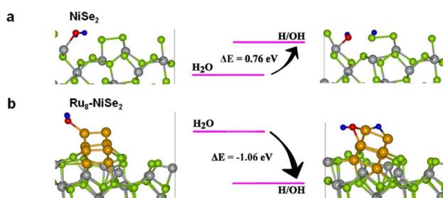
Fig. 7 Representation of reaction pathways. (a) Pristine and (b) Ru<sub>8</sub>-NiSe<sub>2</sub> (210) materials. Green, grey, golden yellow, red, and blue coloured balls represent Se, Ni, Ru, O, and H atoms, respectively.
