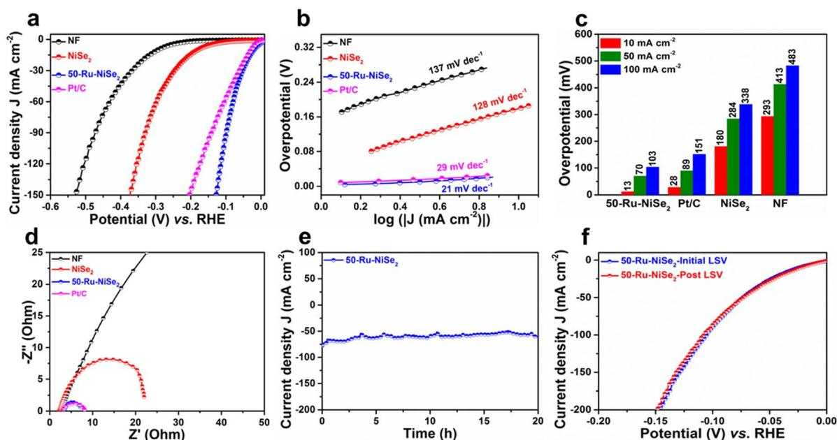
Fig. 3 HER studies. (a) LSV polarization curves recorded for NF, NiSe<sub>2</sub>, 50-Ru-NiSe<sub>2</sub>, and Pt/C. (b) The corresponding Tafel plots. (c) Overpotential measured at current densities of 10, 50, and 100 mA cm<sup>-2</sup>. (d) Comparison of Nyquist plots of NF, NiSe<sub>2</sub>, 50-Ru-NiSe<sub>2</sub> and Pt/C. (e) Stability plot of 50-Ru-NiSe<sub>2</sub> obtained using chronoamperometry measurements. (f) Initial and post LSV plots of 50-Ru-NiSe<sub>2</sub>.
