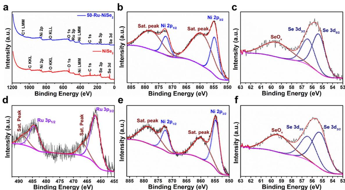
Fig. 2 XPS analysis. (a) Survey spectra of NiSe<sub>2</sub> and 50-Ru-NiSe<sub>2</sub>. (b and c) High-resolution XPS spectra of Ni and Se of NiSe<sub>2</sub>. (d–f) High-resolution XPS spectra of Ru, Ni, and Se of 50-Ru-NiSe<sub>2</sub>.
