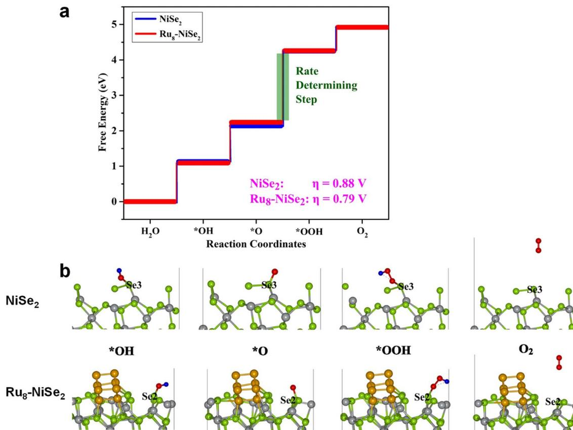
Fig. 8 Theoretical calculations for the OER. (a) Free energy plot and (b) intermediate structures involved in the OER at the minimum overpotential sites of pure and  $\text{Ru}_8\text{-NiSe}_2$  (210) systems.
