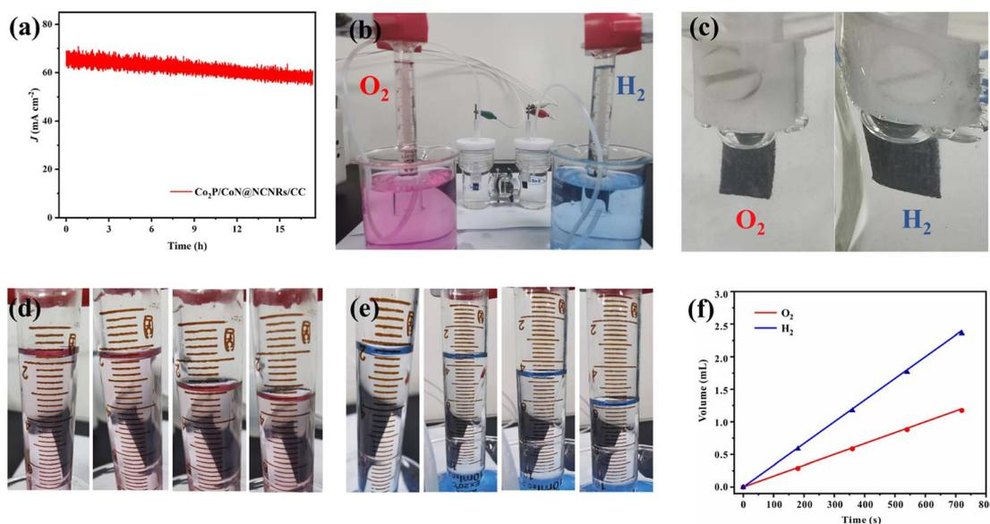
Fig. 9 (a) Long-term durability test of CoP/CoN@NCNRs/CC at 1.65 V, (b) water splitting assembly diagram, (c)  $\text{O}_2$  and  $\text{H}_2$  generation from the anode and cathode, (d and e) linearity of  $\text{O}_2$  and  $\text{H}_2$  production over time, and (f) oxygen and hydrogen generated at 0, 3, 6, 9, and 12 min.
