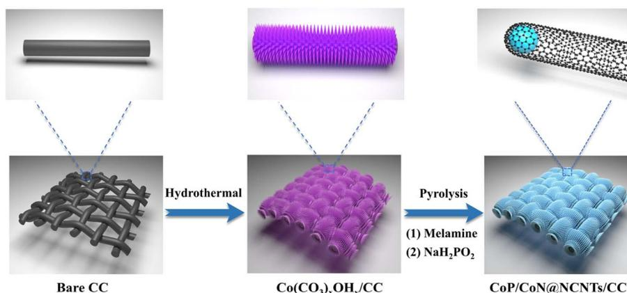
Scheme 1 Illustration for the fabrication of CoP/CoN@NCNRs/CC.
