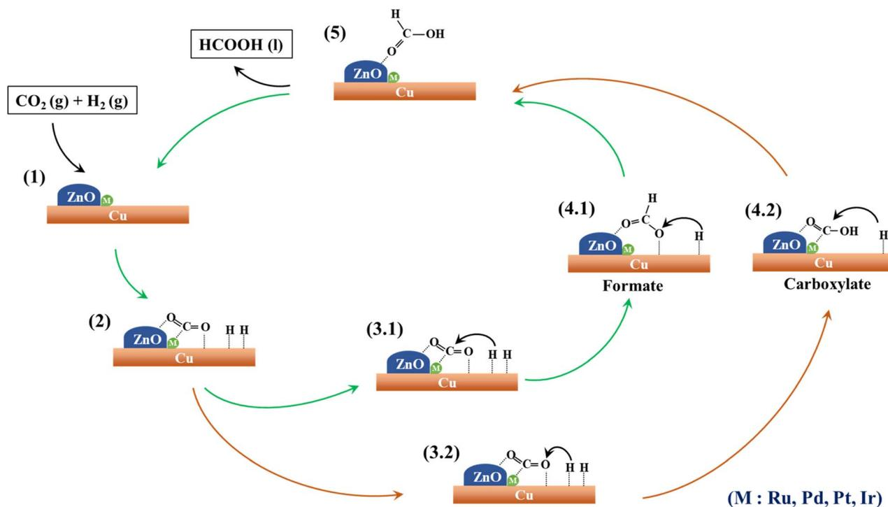
Fig. 9 A proposed mechanism for CO<sub>2</sub> hydrogenation to formic acid over the surface of M–CZ catalysts.
