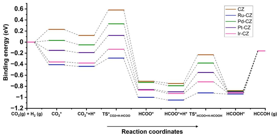
Fig. 19 The energy profile diagram for the hydrogenation of  $\text{CO}_2$  to formic acid on CZ and M-CZ catalyst surfaces.
