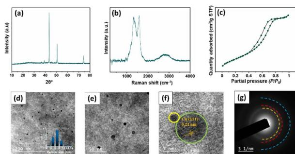
Fig. 8 Characterization of the spent Ru-CZ catalyst. (a) XRD diffractogram, (b) Raman spectroscopy spectra, (c) N<sub>2</sub> isotherm profile, (d-e) TEM images, (f) HR-TEM and (g) SAED.
