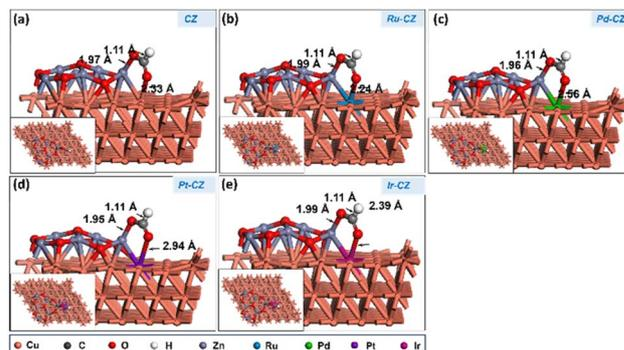
Fig. 13 The DFT optimised geometry of the HCOO adsorption on (a) CZ, (b) Ru-CZ, (c) Pd-CZ, (d) Pt-CZ and (e) Ir-CZ surfaces.
