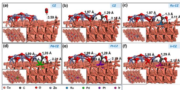
Fig. 11 The DFT optimised geometry of CO<sub>2</sub> adsorption on (a) CZ, (b) CZ, (c) Ru-CZ, (d) Pd-CZ, (e) Pt-CZ and (f) Ir-CZ surfaces.
