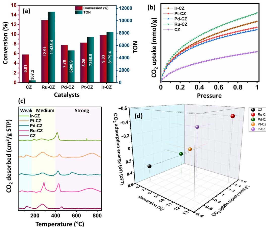
Fig. 6 (a) The performance of various catalysts in CO<sub>2</sub> hydrogenation to formic acid, (b) CO<sub>2</sub> adsorption isotherm at 298 K, (c) CO<sub>2</sub>-TPD profile, (d) CO<sub>2</sub> conversion (%) vs. CO<sub>2</sub> uptake (mmol g<sup>-1</sup>) and CO<sub>2</sub> adsorption energy (DFT) (eV).
