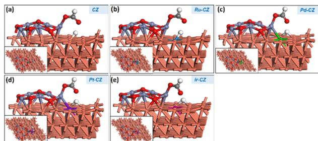
Fig. 17 The geometry optimised structure of the transition state during conversion of  $\text{CO}_2 + \text{H}$  to  $\text{HCOO}$  and  $\text{COOH}$  for (a) CZ, (b) Ru-CZ, (c) Pd-CZ, (d) Pt-CZ and (e) Ir-CZ.
