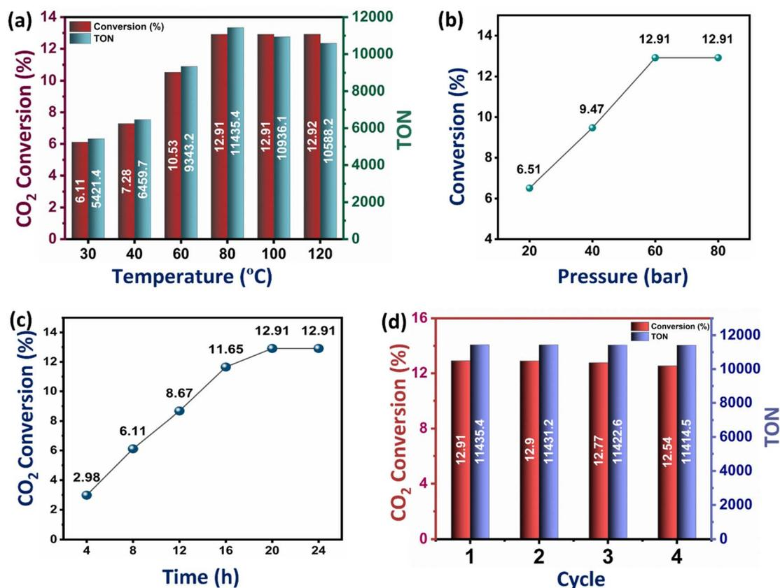
Fig. 7 (a) Effect of temperature on CO<sub>2</sub> conversion and TON for Ru-CZ. (b) Effect of pressure on CO<sub>2</sub> conversion for Ru-CZ. (c) Effect of time on CO<sub>2</sub> conversion for Ru-CZ. (d) Recyclability test for Ru-CZ.
