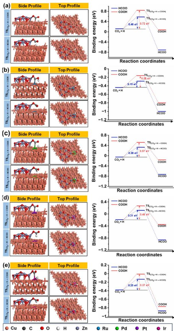
Fig. 15 The geometry optimised structure of the transition state during conversion of  $\text{CO}_2 + \text{H}$  to  $\text{HCOO}$  and  $\text{COOH}$  and associated energy profile diagrams for (a) CZ, (b) Ru-CZ, (c) Pd-CZ, (d) Pt-CZ and (e) Ir-CZ.
