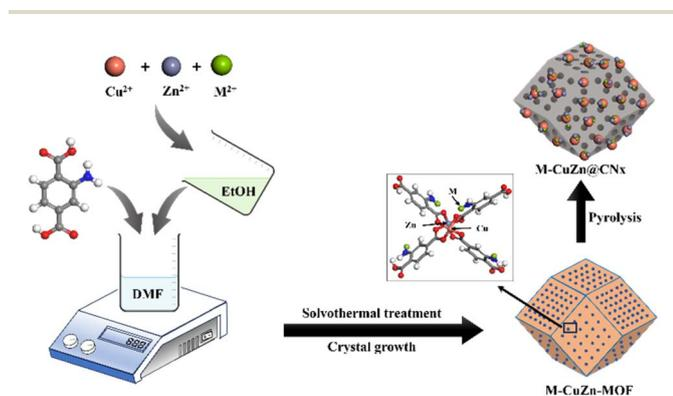
Fig. 1 Schematic representation of the synthesis procedure of M-CuZn@CNx catalysts.
