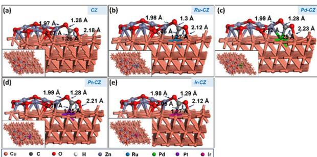
Fig. 12 The DFT optimised geometry of the CO<sub>2</sub> + H co-adsorption on (a) CZ, (b) Ru-CZ, (c) Pd-CZ, (d) Pt-CZ and (e) Ir-CZ surfaces.
