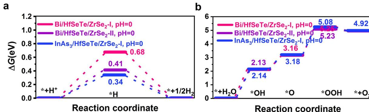
Fig. 8 The Gibbs free energy changes for (a) HERs and (b) OERs at pH = 0 of Bi/HfSeTe/ZrSe<sub>2</sub>-I, Bi/HfSeTe/ZrSe<sub>2</sub>-II, and InAs<sub>3</sub>/HfSeTe/ZrSe<sub>2</sub>-I, respectively.
