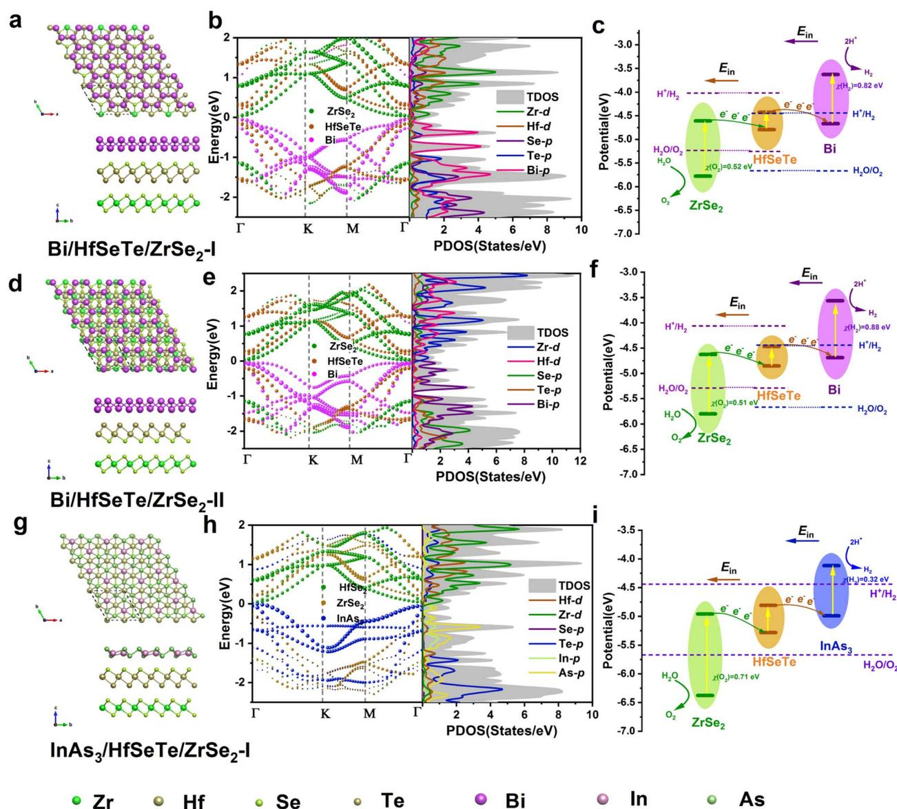
Fig. 3 The geometric structures, band alignments, project density of states, and the schemes for HERs and OERs. (a)–(c) Bi/HfSeTe/ZrSe<sub>2</sub>-I, (d)–(f) Bi/HfSeTe/ZrSe<sub>2</sub>-II, and (g)–(i) InAs<sub>3</sub>/HfSeTe/ZrSe<sub>2</sub>-I.
