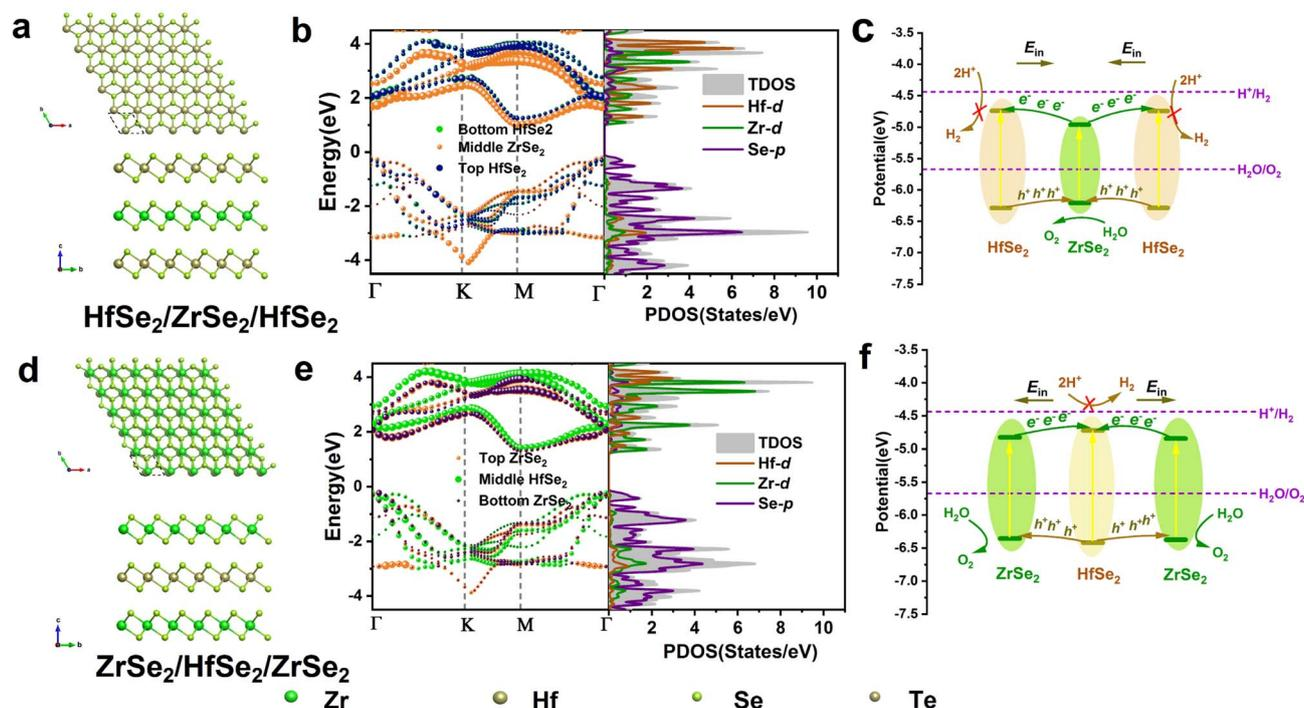
Fig. 1 The geometric structures, band alignments, projected density of states, and the schemes for HERs and OERs. (a)–(c) HfSe<sub>2</sub>/ZrSe<sub>2</sub>/HfSe<sub>2</sub>, and (d)–(f) ZrSe<sub>2</sub>/HfSe<sub>2</sub>/ZrSe<sub>2</sub>.
