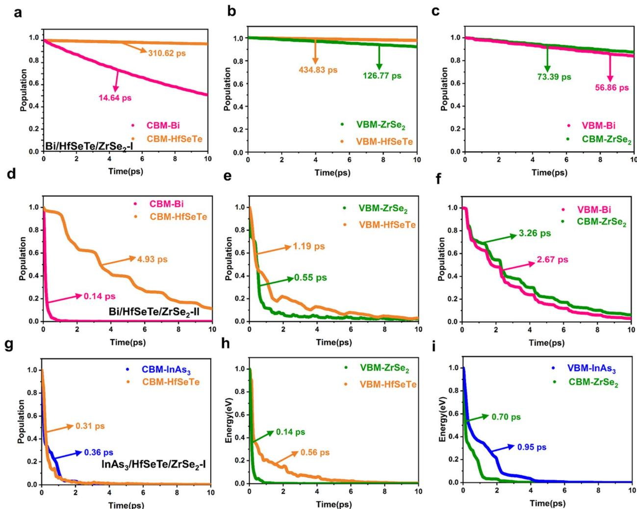
Fig. 7 The carrier transfer dynamics in Bi/HfSeTe/ZrSe<sub>2</sub>-I, Bi/HfSeTe/ZrSe<sub>2</sub>-II, and InAs<sub>3</sub>/HfSeTe/ZrSe<sub>2</sub>-I. (a), (d) and (g) CBM@Bi/InAs<sub>3</sub> and CBM@HfSeTe, (b), (e) and (h) VBM@ZrSe<sub>2</sub> and VBM@HfSeTe, and (c), (f) and (i) CBM@ZrSe<sub>2</sub> and VBM@Bi/InAs<sub>3</sub>.
