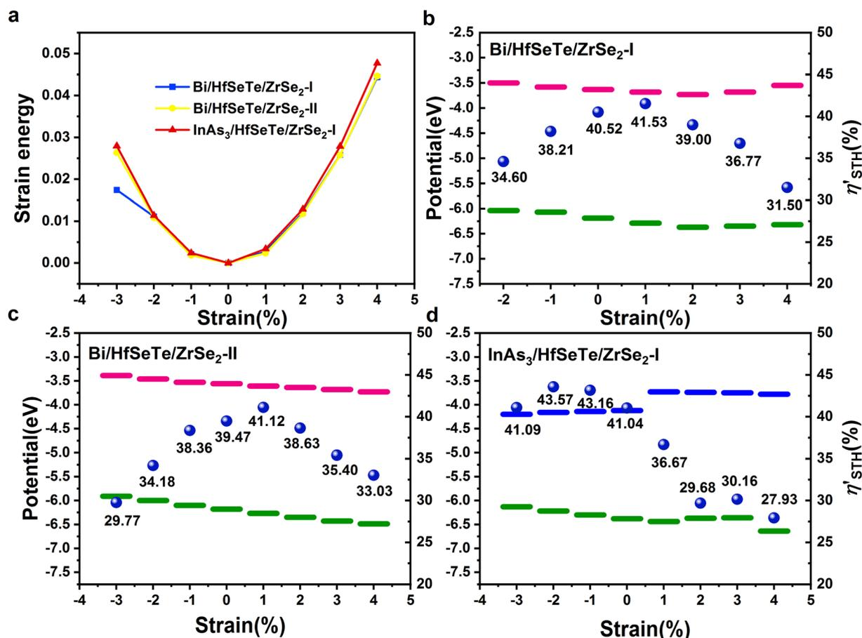
Fig. 4 The strain engineering for heterostructures. (a) The strain energies for Bi/HfSeTe/ZrSe<sub>2</sub>-I, Bi/HfSeTe/ZrSe<sub>2</sub>-II, and InAs<sub>3</sub>/HfSeTe/ZrSe<sub>2</sub>-I. (b)–(d) The potentials of band edges and STH conversion efficiency  $\eta'_{\text{STH}}$  of Bi/HfSeTe/ZrSe<sub>2</sub>-I, Bi/HfSeTe/ZrSe<sub>2</sub>-II, and InAs<sub>3</sub>/HfSeTe/ZrSe<sub>2</sub>-I under biaxial strains. The blue balls represent  $\eta'_{\text{STH}}$ .
