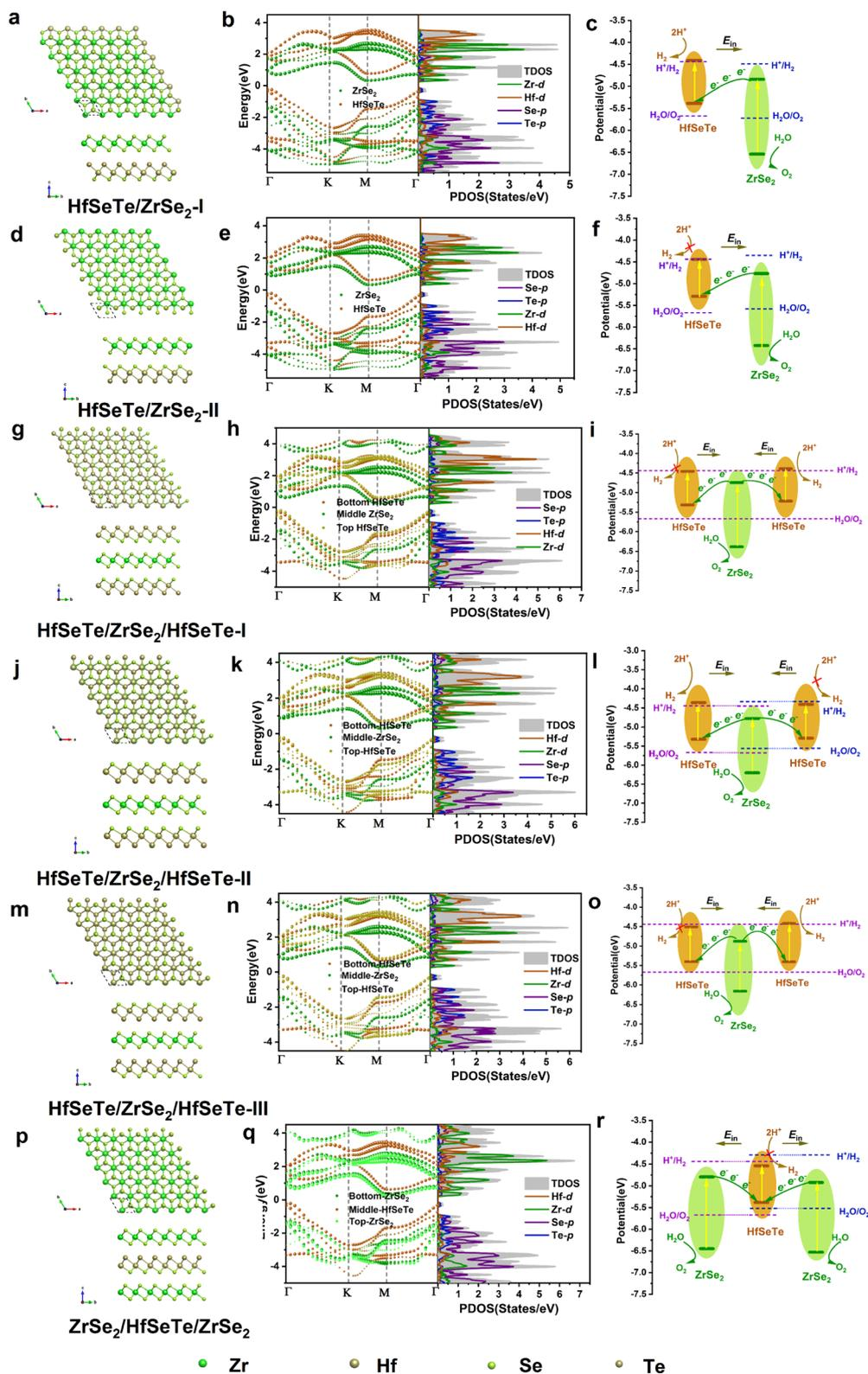
Fig. 2 The geometric structures, band alignments, project density of states, and the schemes for HERs and OERs. (a)–(c) HfSeTe/ZrSe<sub>2</sub>-I, (d)–(f) HfSeTe/ZrSe<sub>2</sub>-II, (g)–(i) HfSeTe/ZrSe<sub>2</sub>/HfSeTe-I, (j)–(l) HfSeTe/ZrSe<sub>2</sub>/HfSeTe-II, (m)–(o) HfSeTe/ZrSe<sub>2</sub>/HfSeTe-III, and (p)–(r) ZrSe<sub>2</sub>/HfSeTe/ZrSe<sub>2</sub>.
