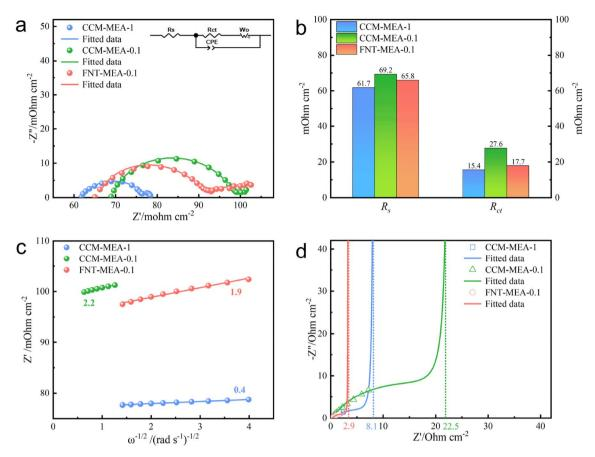
Fig. 4 (a) Nyquist plots of the CCM-MEAs and FNT-MEA at 1.6 V vs. DHE. The inset shows an equivalent circuit. (b) The ohmic resistance ( $R_{cl}$ ) and charge transfer resistance ( $R_{ct}$ ) of the CCM-MEAs and FNT-MEA. (c) Weber coefficient of the CCM-MEAs and FNT-MEA, which can reflect mass transfer at high potential. (d) Nyquist plots of the ACL for CCM-MEAs and FNT-MEA under  $H_2/N_2$  conditions.
