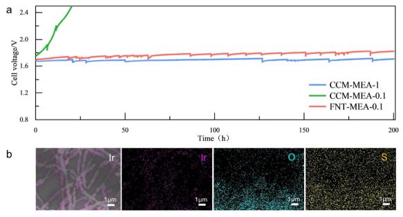
Fig. 5 (a) The stability test of the CCM-MEAs and FNT-MEA at 1 A cm<sup>-2</sup> and 65 °C. (b) The corresponding EDS-mapping after the durability test.
