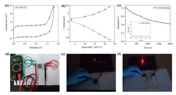
Fig. 6 (a) CV loops obtained from the supercapacitor, (b) current vs. square root of scan rate, and (c) OCP of devices fabricated using TBFT1 in the dropcast form. Photographs of the ECD (d) connected to a multimeter after withdrawing the externally applied current, (e and f) during discharging (LED light on) test; the two ECDs in the gel state were connected in series.
