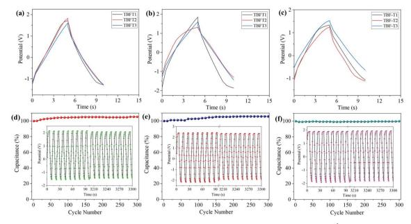
Fig. 7 Galvanostatic charge-discharge curves of the supercapacitors TBFT1-3 (at a current density of 10 A g<sup>-1</sup>) in the (a) gel state, (b) dropcast form, and (c) dropcast form with a Nafion coating. Cycling stability (300 cycles of continuous charging and discharging) of the supercapacitors derived from TBFT1 in the (d) gel state (c.d. 20 A g<sup>-1</sup>), (e) dropcast form (c.d. 10 A g<sup>-1</sup>), and (f) dropcast form with a Nafion coating (50 A g<sup>-1</sup>).
