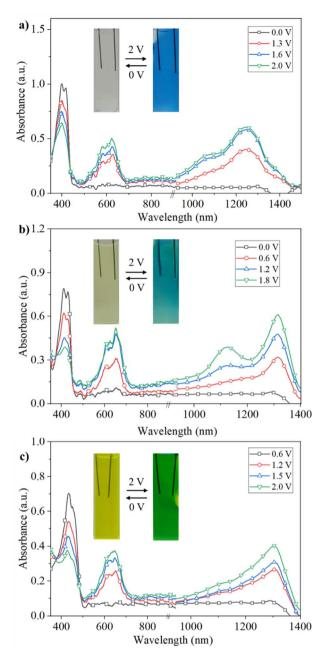
Fig. 3 Spectroelectrochemistry of (a) TBFT1, (b) TBFT2, and (c) TBFT3 in 0.1 M TBAPF<sub>6</sub> in DCM at applied potentials carried out with a Pt mesh working electrode, Pt wire counter electrode, and Ag/Ag+ quasi reference electrode.
