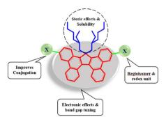
Fig. 1 The design strategy of electrochromic tetrabenzofluorene derivatives via band gap tuning by increasing conjugation, anchoring with thiophene derivatives, and improving the solubility by incorporating branched alkyl groups.
