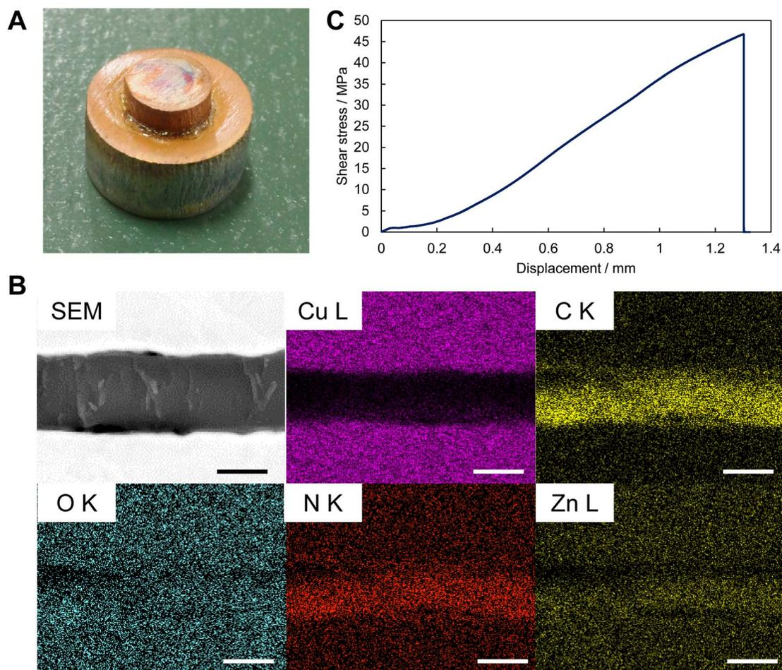
Fig. 4 Adhesive characterization of the ZIF-zni gel. (A) Photograph of the adhesive body. (B) Cross-sectional SEM image and EDX analysis of the adhesive body. Scale bar: 1  $\mu\text{m}$ . (C) Stress-displacement curve of the adhesive body.
