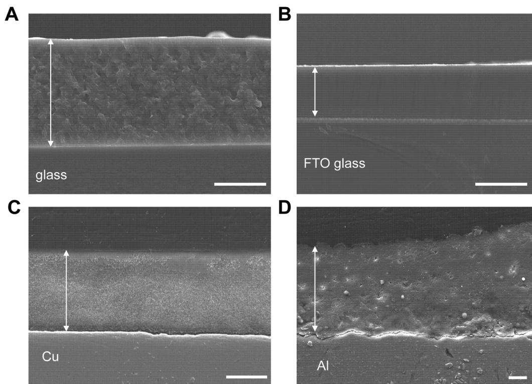
Fig. 2 Cross-sectional SEM images of ZIF-zni films on different substrates. (A) Glass. (B) FTO glass. (C) Cu. (D) Al. Scale bars: 5  $\mu\text{m}$ .
