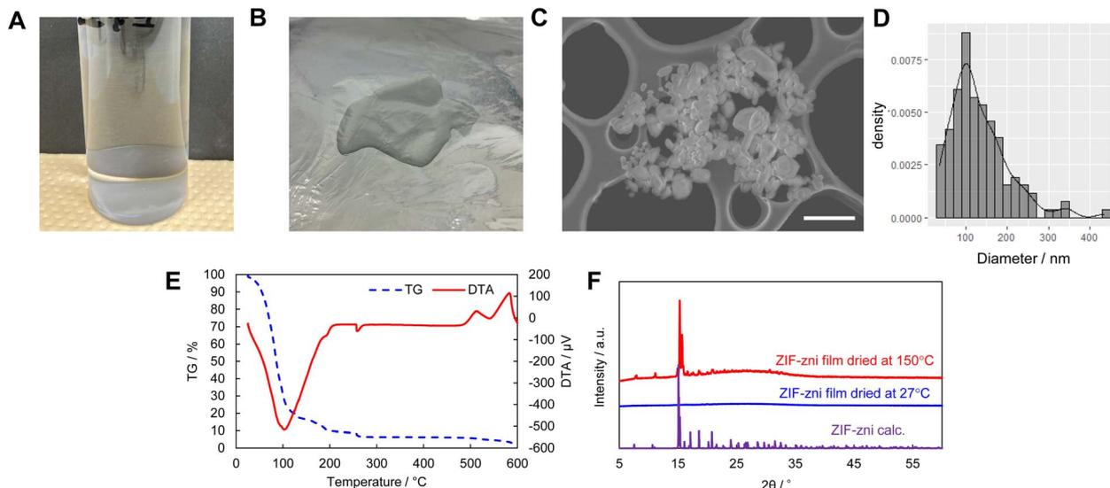
Fig. 1 Characterization of the ZIF-zni gel. (A) ZIF-zni colloidal solution. (B) ZIF-zni gel. (C) SEM images of ZIF-zni particles (scale bar: 1  $\mu\text{m}$ ). (D) Particle size distribution of the ZIF-zni gel. (E) Thermogravimetric analysis of the ZIF-zni gel. (F) XRD patterns of the ZIF-zni films.
