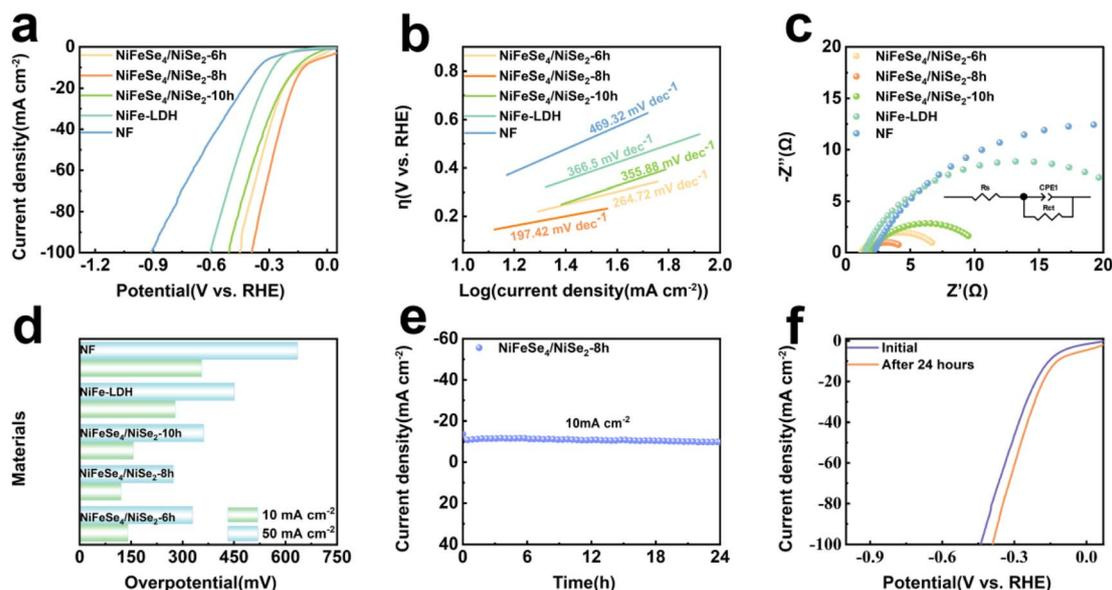
Fig. 6 HER performance of the catalytic electrodes NF, NiFe-LDH, NiFeSe<sub>4</sub>/NiSe<sub>2</sub>-6 h, NiFeSe<sub>4</sub>/NiSe<sub>2</sub>-8 h and NiFeSe<sub>4</sub>/NiSe<sub>2</sub>-10 h: (a) LSV curves; (b) Tafel diagram; (c) Nyquist diagram; (d) different current densities corresponding to overpotential; (e) stability test diagram; (f) performance comparison diagram before and after reaction.
