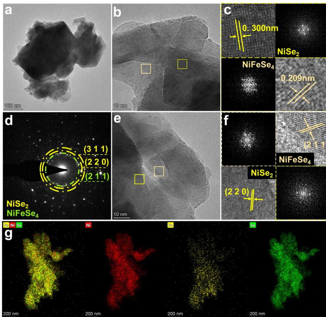
Fig. 3 (a) The NiFeSe<sub>4</sub>/NiSe<sub>2</sub>-8 h heterostructure stripped from NF and (b) its corresponding HRTEM image; (c) HRTEM corresponding lattice fringes and its FFT pattern; (d) SAED pattern of NiFeSe<sub>4</sub>/NiSe<sub>2</sub>-8 h; (e) image at the NiFeSe<sub>4</sub>/NiSe<sub>2</sub>-8 h interface and (f) lattice fringes at the interface; (g) EDS mapping image.
