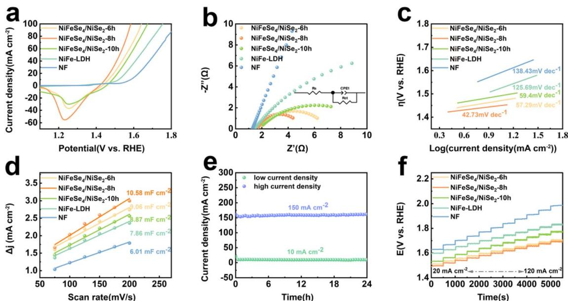
Fig. 5 OER performance of catalytic electrodes NF, NiFe-LDH, NiFeSe<sub>4</sub>/NiSe<sub>2</sub>-6 h, NiFeSe<sub>4</sub>/NiSe<sub>2</sub>-8 h and NiFeSe<sub>4</sub>/NiSe<sub>2</sub>-10 h: (a) LSV curves; (b) Nyquist diagram; (c) Tafel diagram; (d)  $C_{dl}$  measurement; (e) stability tests at high and low current densities; (f) multi-potential step.
