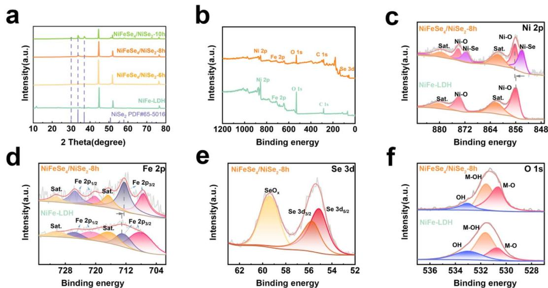
Fig. 4 (a) XRD patterns of NiFe-LDH, NiFeSe<sub>4</sub>/NiSe<sub>2</sub>-6 h, NiFeSe<sub>4</sub>/NiSe<sub>2</sub>-8 h, and NiFeSe<sub>4</sub>/NiSe<sub>2</sub>-10 h; (b) the high-resolution XPS spectra of (c) Ni 2p, (d) Fe 2p, (e) Se 3d and (f) O 1s of NiFe-LDH and NiFeSe<sub>4</sub>/NiSe<sub>2</sub>-8 h.
