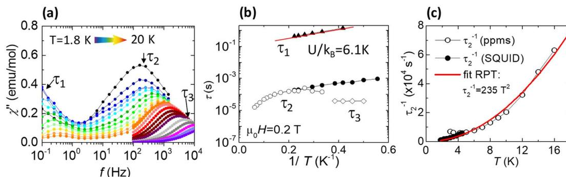
Fig. 5 (a) Imaginary component of the ac susceptibility as a function of the frequency,  $\chi''(f)$ , of complex **1** at  $\mu_0 H = 0.2$  T and different temperatures ranging from 1.8 K to 20 K; (b) magnetic relaxation time as a function of the inverse temperature ( $1/T$ ) at  $\mu_0 H = 0.2$  T; (c) temperature dependence of  $\tau_2^{-1}(T)$ , and a fit to a power law  $\tau_2^{-1} = KT^2$ , with  $K = 235$  s $^{-1}$  K $^{-2}$  between 2–16 K.
