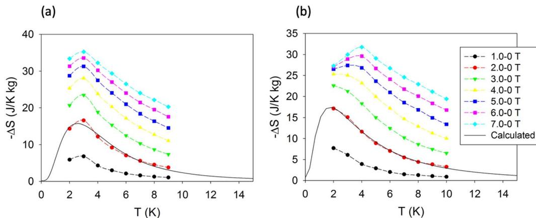
Fig. 8 Magnetic entropy change,  $-\Delta S_m$ , for **1** grafted on a TSP functionalized Si wafer, **1Si**, with the wafer parallel (a) and perpendicular (b) to the SQUID magnetic field. The solid line is a mathematical fit to a logarithmic peak function.
