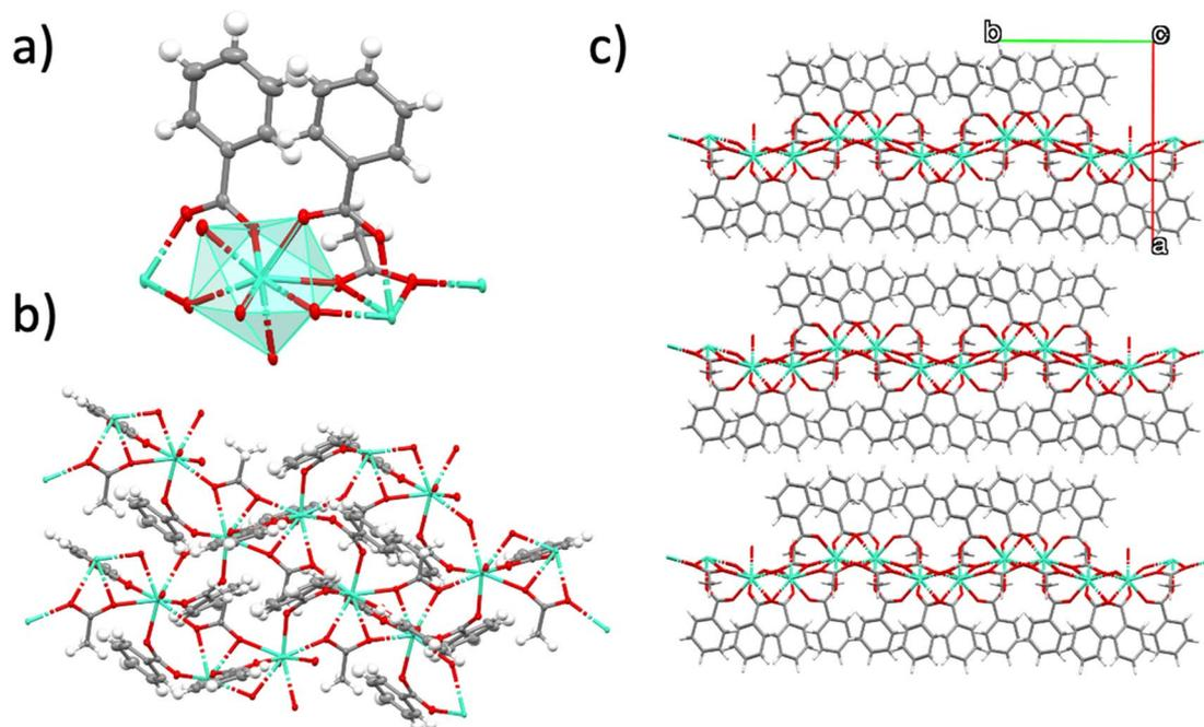
Fig. 1 Crystal structure of **1**. (a) A fragment of **1** showing thermal ellipsoids (50%) and with a polyhedral representation for Gd1; (b) top view of the 2D layer of **1**; (c) crystal packing along the *a*-axis of the unit cell. The crystal packing shows a stack of three layers of **1** with only van der Waals interactions between them. Gd: green; C: grey; O: red; H: white.
