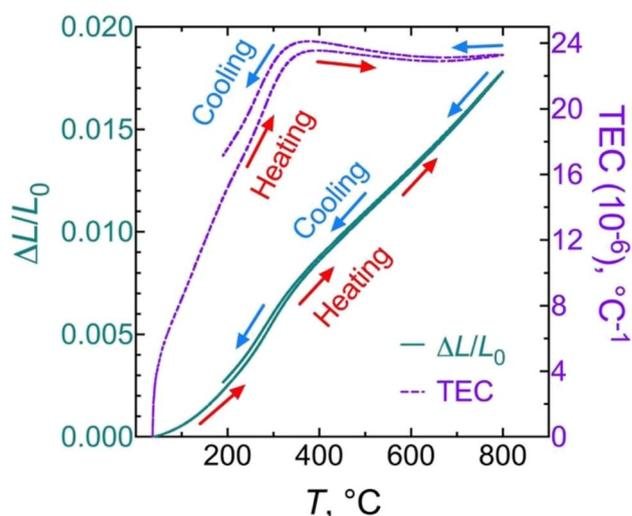
Fig. 4 Linear thermal expansion/shrinkage (left) and thermal expansion coefficient (TEC) (right) of the Ba<sub>2</sub>Co<sub>9</sub>O<sub>14</sub> ceramic.
