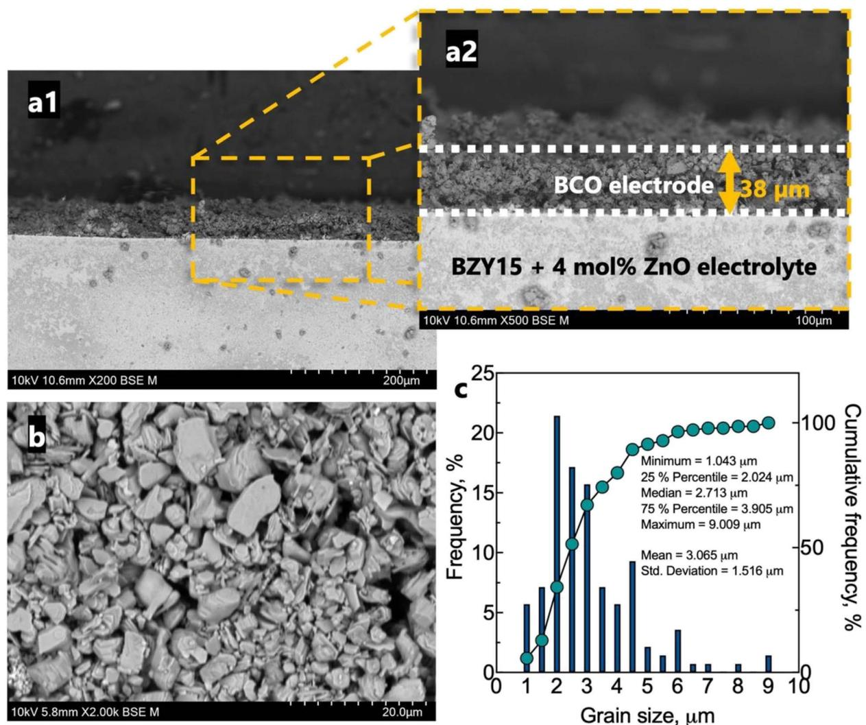
Fig. 5 Microstructure of the electrochemical cell after tests: (a) cross section of the BCO-BZY15 + 4 mol% ZnO half cell; (b) top view of the BCO electrode; (c) relative/cumulative frequency histogram of the grain size distribution.
