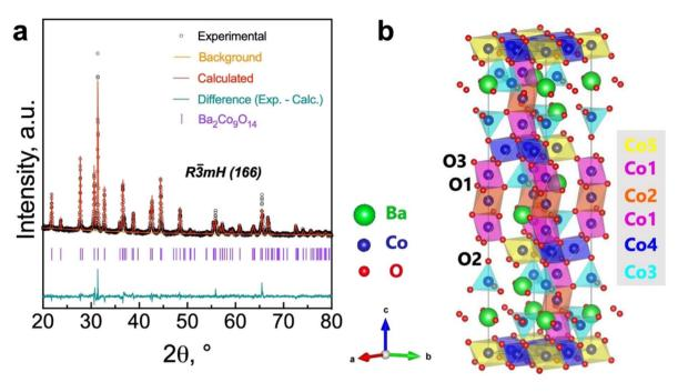
Fig. 2 Rietveld refinement of the  $Ba_2Co_9O_{14}$  oxide: (a) room temperature XRD pattern; (b) crystal structure.
