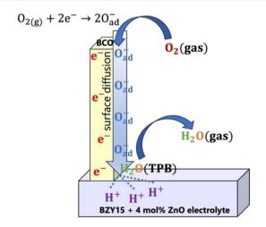
Fig. 8 Schematic of the possible reaction steps for the Ba<sub>2</sub>Co<sub>9</sub>O<sub>14</sub> cathode
