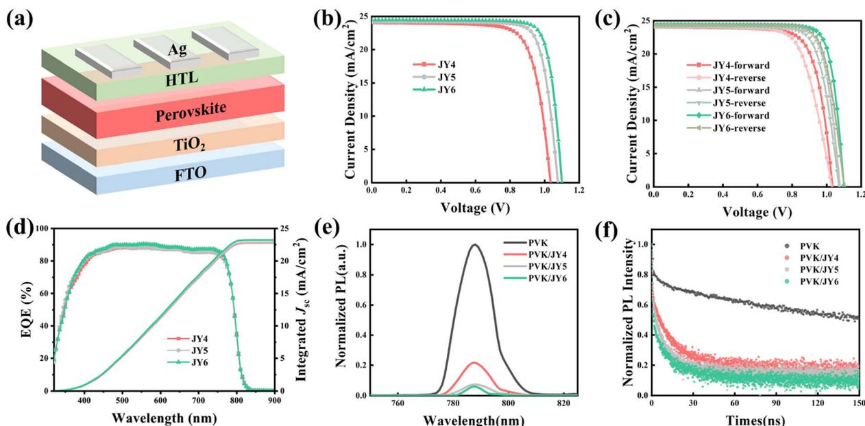
Fig. 8 (a) PSC device assembly diagram. (b)  $J$ - $V$  curves of JY4, JY5, and JY6 based PSC devices. (c)  $J$ - $V$  curves under reverse and forward scans for JY4, JY5, and JY6. (d) EQE and integrated  $J_{sc}$  of the JY4–JY6 based PSCs. (e) Steady-state PL spectra of the perovskite films, and JY4, JY5, and JY6 films on the perovskites. (f) Time-resolved PL decay of the perovskite films, and JY4, JY5, and JY6 films on the perovskites.
