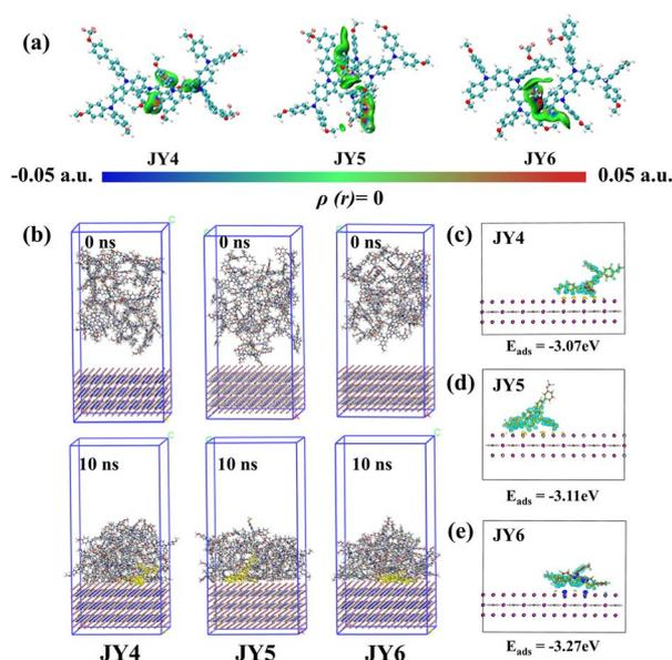
**Fig. 4** (a) IGM analysis based on the original molecular density shows the weak interaction of the designed HTM dimer. All iso-surfaces (isovalue = 0.001) are colored for the promolecular density range of  $-0.05 < \rho(r) < 0.05$  a.u. (b) The distribution of HTMs on the perovskite surface after 10 ns is simulated by the MD method. (c–e) Adsorption energy of the perovskite surface to the HTM and electron charge density differences.
