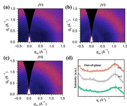
Fig. 6 The GIWAXS images of (a) JY4, (b) JY5 and (c) JY6. (d) The corresponding line cuts from GIWAXS patterns for JY4–JY6.
