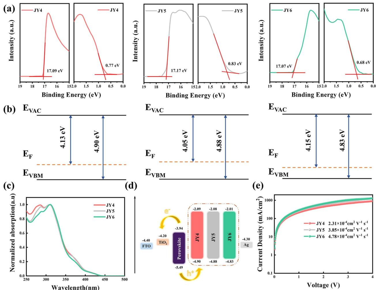
Fig. 5 (a) UPS spectra of the JY4–JY6 films (b) energy diagram for JY4–JY6. (c) Measured absorption spectra of JY4, JY5, and JY6. (d) Energy levels of JY4, JY5, and JY6 in PSC devices. (e) Dark  $J$ - $V$  curves of JY4, JY5, and JY6 for measurement of hole mobility.
