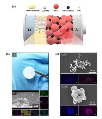
Fig. 1 (a) Illustration of an ASSLSeB comprising a CPE and a Se/C cathode. (b) (i) Visual image of a polyethylene oxide (PEO)/LLZANO/ LiTFSI/SN-CPE disk; (ii) CPE surface morphology and elemental mapping by energy dispersive X-ray spectroscopy (EDS). (c) Micromorphologies and EDS elemental mapping results of Se/KB and Se/ MPC cathode materials.
