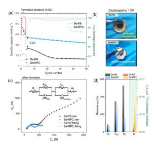
**Fig. 2** Comparison of Se/KB and Se/MPC cathode behavior. (a) Se/KB and Se/MPC capacities at 0.2C as a function of cycle number after a 3-cycle, 0.05C formation protocol. (b) Optical image of CPE in cells after discharge to 1.0 V. (c) Nyquist plots of Se/KB and Se/MPC cells after formation; the inset contains an equivalent circuit for the fitting. (d) Resistance parameters (R) and Li<sup>+</sup> diffusion coefficient ( $D_{Li^+}$ ) obtained by EIS.
