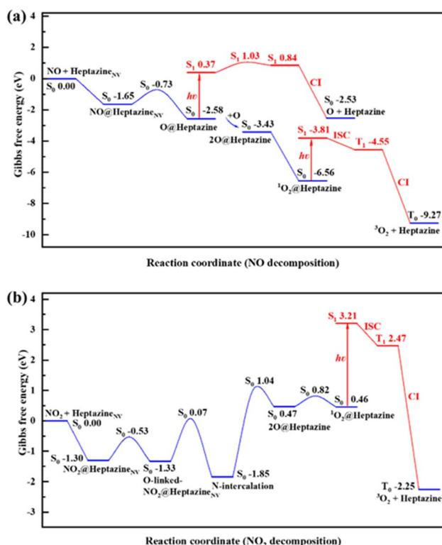
Fig. 5 Gibbs free energy profiles of (a) NO and (b)  $NO_2$  decompositions on heptazine<sub>NV</sub> at  $T = 300$  K and  $P = 1.00$  atm by  $\omega$ B97XD/6-31G(d,p) calculations. The free energy values relative to the initial reactants of NO/ $NO_2$  and heptazine<sub>NV</sub> are labelled to indicate the barrier ( $G_b$ ) and change ( $\Delta G$ ) for each step.
