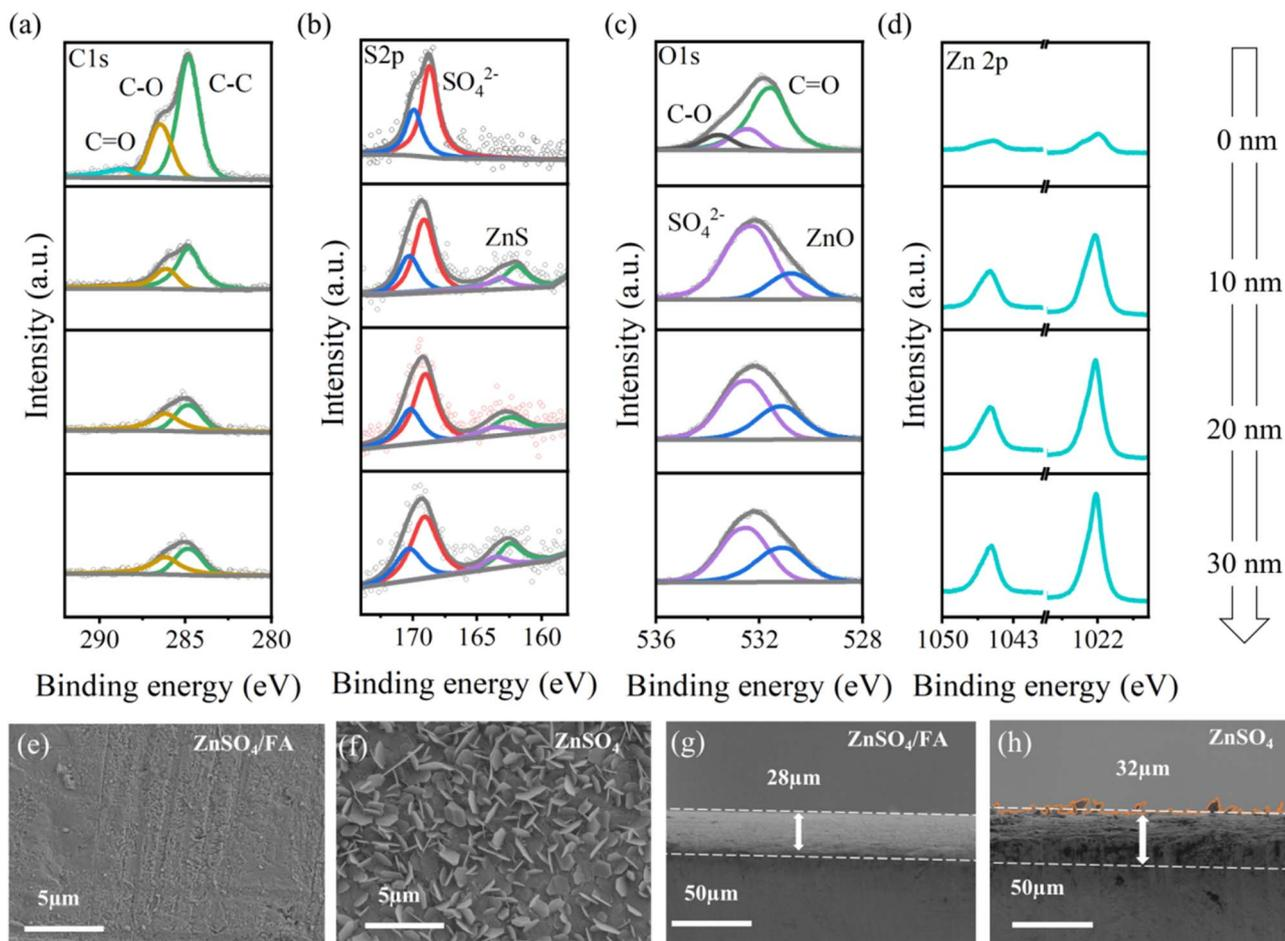
Fig. 3 (a–d) XPS depth profile of the Zn anode after 25 plating/stripping cycles in ZnSO<sub>4</sub>/FA electrolyte at a current density of 1 mA cm<sup>-2</sup> with a capacity of 0.5 mA h cm<sup>-2</sup>. (e and f) The plan-view and (g and h) cross section SEM images of the Zn anode after a plating/stripping cycle in (e and g) ZnSO<sub>4</sub>/FA electrolyte and (f and h) pure ZnSO<sub>4</sub> electrolyte at a current density of 1 mA cm<sup>-2</sup> with a capacity of 0.5 mA h cm<sup>-2</sup>.
