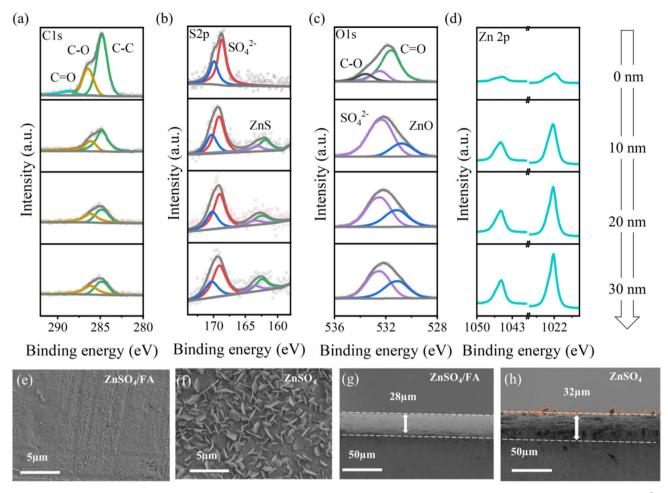
Fig. 3 (a-d) XPS depth profile of the Zn anode after 25 plating/stripping cycles in  $ZnSO_4/FA$  electrolyte at a current density of 1 mA cm<sup>-2</sup> with a capacity of 0.5 mA h cm<sup>-2</sup>. (e and f) The plan-view and (q and h) cross section SEM images of the Zn anode after a plating/stripping cycle in (e and g) ZnSO<sub>4</sub>/FA electrolyte and (f and h) pure ZnSO<sub>4</sub> electrolyte at a current density of 1 mA cm<sup>-2</sup> with a capacity of 0.5 mA h cm<sup>-1</sup>
