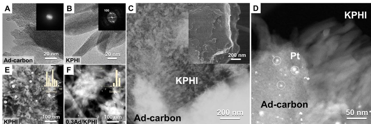
Fig. 4 TEM images of (A) Ad-carbon and (B) KPHI. High angle annular dark-field (HAADF)-STEM images of 3Ad/KPHI (C) before and (D) after 6 h of the H<sub>2</sub> evolution reaction. (In order to locate the Ad-carbon/KPHI heterojunction more easily during STEM observation, we prepared a hybrid sample with 10× the concentration of 0.3Ad/KPHI.) HAADF-STEM images of (E) KPHI and (F) 0.3Ad/KPHI with photodeposited Pt nanoparticles.
