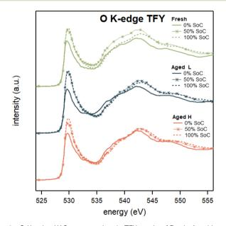
Fig. 6 O K-edge XAS spectra taken in TFY mode of Fresh, Aged L, and Aged H samples in 0, 50 and 100% SoC.
