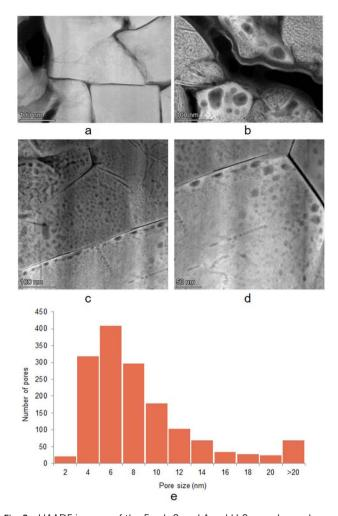
Fig. 2 HAADF images of the Fresh 0 and Aged H 0 samples and pore distribution histogram: (a) HAADF images of Fresh 0 NCA primary particles within the electrode; (b-d) HAADF images of Aged H primary particles within the electrode. The pore size distribution histogram derived from the Aged H 0 image analysis (e).
