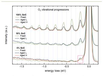
Fig. 8 O K-edge RIXS spectra displaying the region of O<sub>2</sub> vibrations. The spectra are integrated over the excitation energies 531.2-533.2 eV. The red box highlights the difference between Fresh, Aged L, and Aged H samples at 0% SoC.
