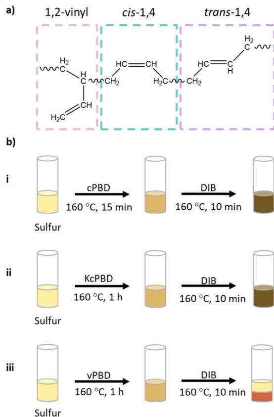
Fig. 1 (a) Displays the three microstructures, 1,2-vinyl, *cis*-1,4 and *trans*-1,4 of PBD; (b) shows a representation of the colour changes during, (i) reaction of sulfur, cPBBD and DIB, (ii) sulfur, KcPBBD, and DIB with the reaction mixtures darkening as the viscosity increases, whereas (iii) reaction of sulfur, vPBBD and DIB shows a separation in the reaction mixture.
