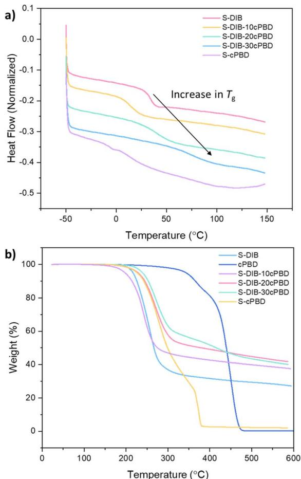
Fig. 3 (a) DSC of S-DIB, S-cPBD, and samples with 10–30 wt% cPBD loadings showing the effect of an increase in cPBD loading on the  $T_g$ ; (b) TGA of the same samples including neat cPBD in addition, displaying the effect of an increase in cPBD loading on the onset decomposition temperature.
