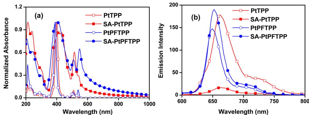
Fig. 2 (a) Absorption and (b) emission spectra of Pt(II)-porphyrins recorded in THF (10  $\mu$ M) and SA Pt(II)-porphyrins recorded in H<sub>2</sub>O at room temperature under argon.
