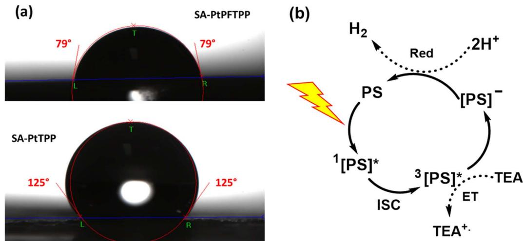
Fig. 7  $\text{H}_2\text{O}$  contact angle measurements of (a) SA-PtPFTPP and SA-PtTPP in  $\text{H}_2\text{O}$  and (b) proposed cyclic PHE mechanism of SA Pt(II)-porphyrins (PS = SA Pt(II)-porphyrins, ET = electron transfer and Red = reduction).
