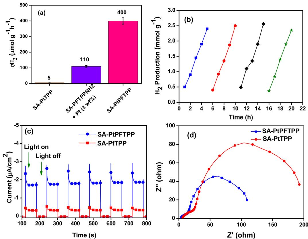
Fig. 6 (a)  $\eta_{H_2}$  of photocatalytic systems of SA-PtPFTPP, SA-PtTPP and SA-PFTPPNH<sub>2</sub> under irradiation for 5 h (3 wt% Pt cocatalyst was added in the case of SA-PFTPPNH<sub>2</sub>), (b) H<sub>2</sub> production of different cycles of the SA-PtPFTPP photocatalytic system, (c) photocurrent–time response spectra of SA-PtPFTPP and SA-PtTPP and (d) Nyquist plots of SA-PtPFTPP and SA-PtTPP under illumination conditions.
