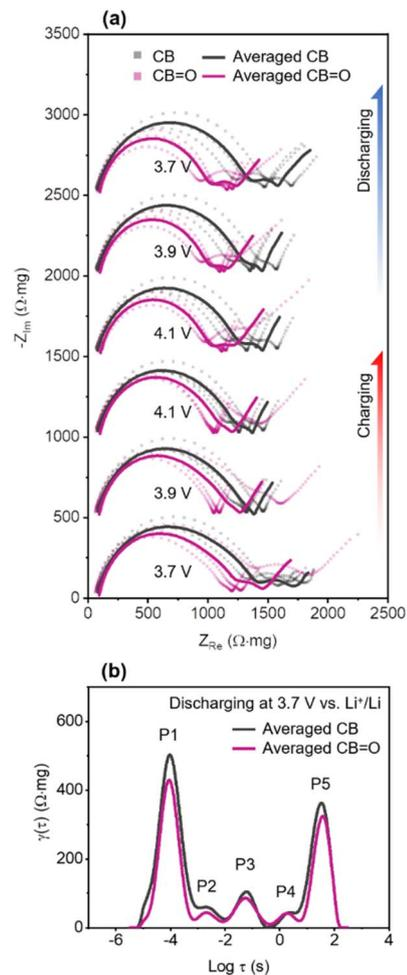
**Fig. 4** (a) Nyquist plots of pristine CB and CB=O (72 h) at 3.7, 3.9, and 4.1 V vs.  $\text{Li}^+/\text{Li}$  during charging and discharging. The dotted lines denote measurement of individual cells and solid lines are averages. (b) Distribution of relaxation times (DRT) of averaged pristine CB and CB=O (72 h) at 3.7 V vs.  $\text{Li}^+/\text{Li}$  discharging.
