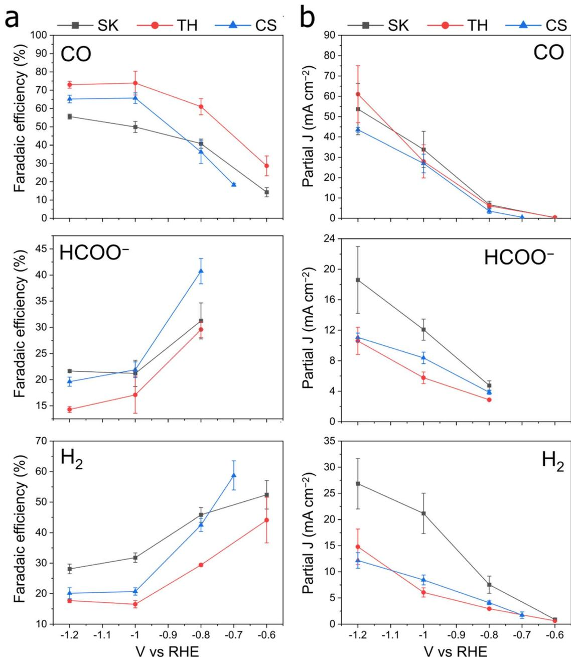
Fig. 4 Electrochemical CO<sub>2</sub>RR performance of catalysts. Data for (a) faradaic efficiency and (b) current density. The electrolyte used was 1 M KHCO<sub>3</sub>. Data were collected from three individual experiments each, and the error bars represent the standard deviation. The data are displayed for CO, HCOO<sup>-</sup> and H<sub>2</sub>.
