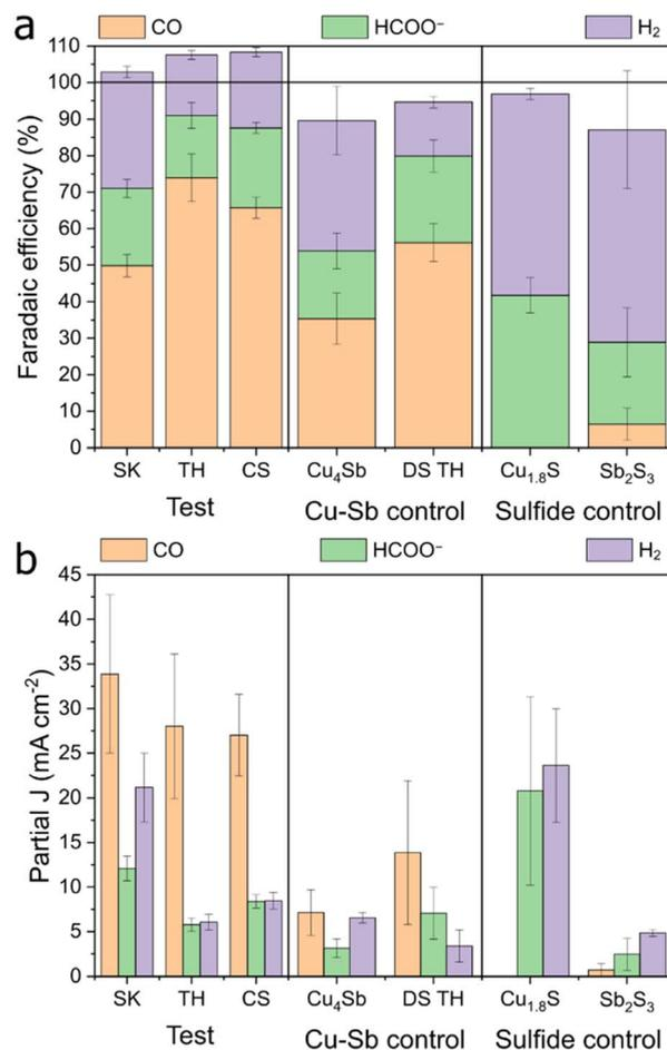
Fig. 3 Electrochemical CO<sub>2</sub>RR performance of the test vs. control (Cu–Sb or sulfide) samples at  $-1.0$  V vs. RHE. Data for (a) faradaic efficiency and (b) current density. The electrolyte used was 1 M KHCO<sub>3</sub>. For the test samples, data were collected from three individual experiments each, and the error bars represent the standard deviation.
