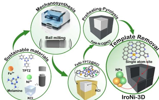
Fig. 1 Schematic illustration of the template-assisted mechanochemistry process.
