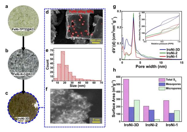
Fig. 2 (a-c) IroNi-3d at different processing stages; (d) SEM image of IroNi-3d; (e) particle size distribution of FeNi nanoparticles in IroNi-3d; (f) HR-STEM image of IroNi-3d; (g) pore size distribution curves and nitrogen adsorption—desorption isotherms (inset). (h) Pore surface area ratio in all three samples.
