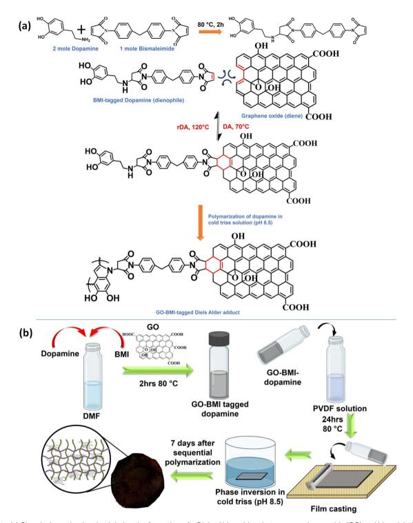
Scheme 1 (a) Chemical reaction involved during the formation of a Diels-Alder adduct between graphene oxide (GO) and bismaleimide (BMI). (b) A cartoon depicting the sequential IPN membrane fabrication process.
