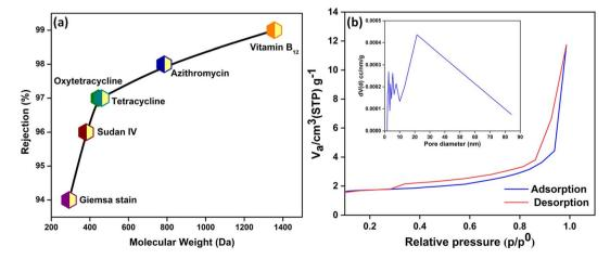
Fig. 3 (a) Molecular weight cut-off analysis of the m-IPN membrane using a range of neutral solutes and (b) pore size analysis from the N₂ adsorption-desorption isotherm.
