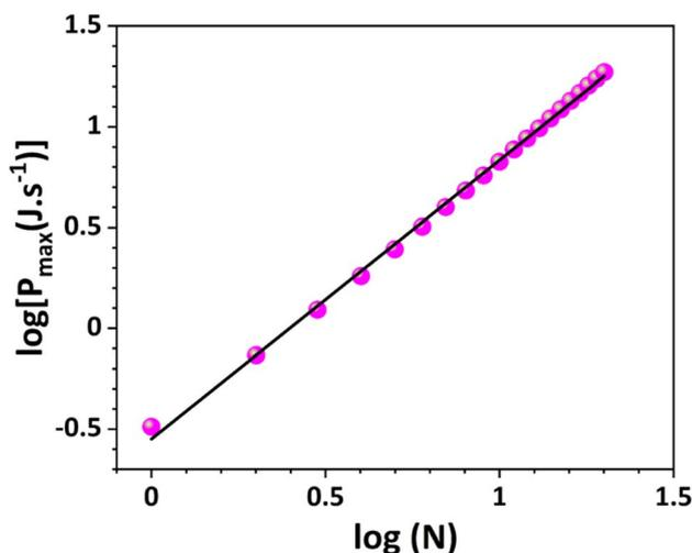
Fig. 12 Maximum power vs.  $N$  two-level systems. By linear fitting, we have obtained  $\alpha = 1.4$ .
