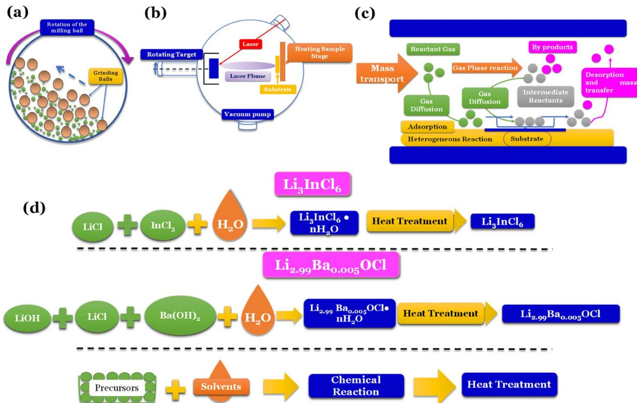
Fig. 5 Synthesis methods: (a) high energy density ball milling;<sup>76</sup> (b) pulsed laser deposition (PLD);<sup>77</sup> (c) chemical vapor deposition (CVD);<sup>78</sup> (d) water mediated synthesis of  $\text{Li}_3\text{InCl}_6$ ,<sup>41</sup>  $\text{Li}_{2.99}\text{Ba}_{0.005}\text{OCl}$ ,<sup>29</sup>  $\text{K}_{2.99}\text{Ba}_{0.005}\text{OCl}$  and  $\text{Na}_{2.99}\text{Ba}_{0.005}\text{OCl}$ .<sup>28</sup>
