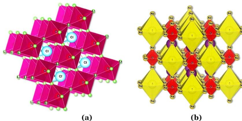
Fig. 7 Antiperovskite electrolytes structures: (a)  $\text{Li}_3\text{OCl}$ ;<sup>29</sup> (b)  $\text{Li}_6\text{SO}(\text{BH}_4)_2$ .<sup>91</sup> CIF files: ref. 53–66.
