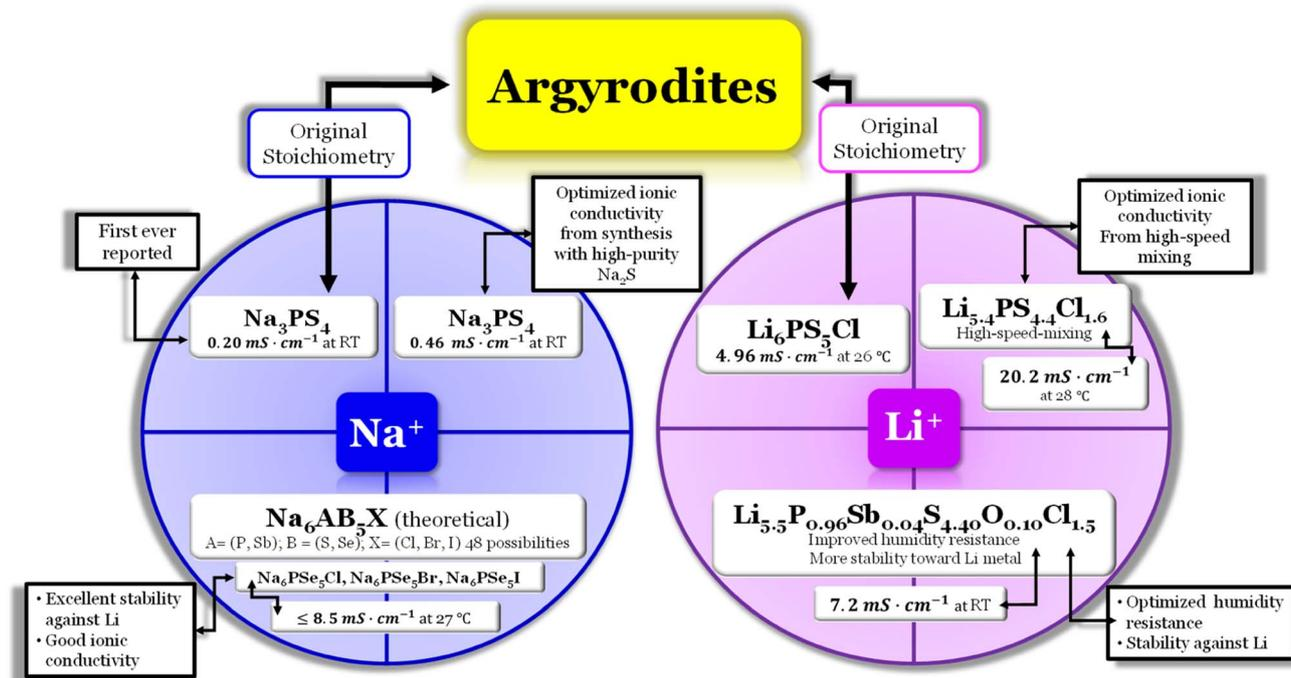
Fig. 6 Argyrodite summary scheme, Li<sub>6</sub>PS<sub>5</sub>Cl,<sup>14</sup> Li<sub>5.4</sub>PS<sub>4.4</sub>Cl<sub>1.6</sub>,<sup>30</sup> Li<sub>5.5</sub>P<sub>0.96</sub>Sb<sub>0.04</sub>S<sub>4.40</sub>O<sub>0.10</sub>Cl<sub>1.5</sub>,<sup>83</sup> Na<sub>3</sub>PS<sub>4</sub>,<sup>84,85</sup> and Na<sub>6</sub>AB<sub>5</sub>X, A = (P, Sb), B = (S, Se), and X = (Cl, Br, I).<sup>86</sup>
