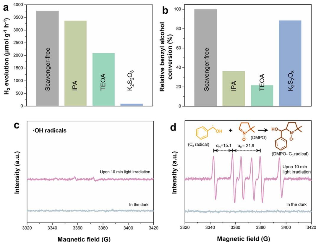
Fig. 6 Scavenger tests for the (a) H<sub>2</sub> evolution rate and (b) benzyl alcohol conversion. Conversion rates are normalized to 100% based on the scavenger-free sample. Condition: scavenger was added same as the mole of benzyl alcohol added. EPR spectra of (c) hydroxyl (·OH) radicals and (d) carbon-centered (·CH(OH)Ph) radicals under light irradiation over LZIS-4. The spectra are recorded at 10 min light illumination.
