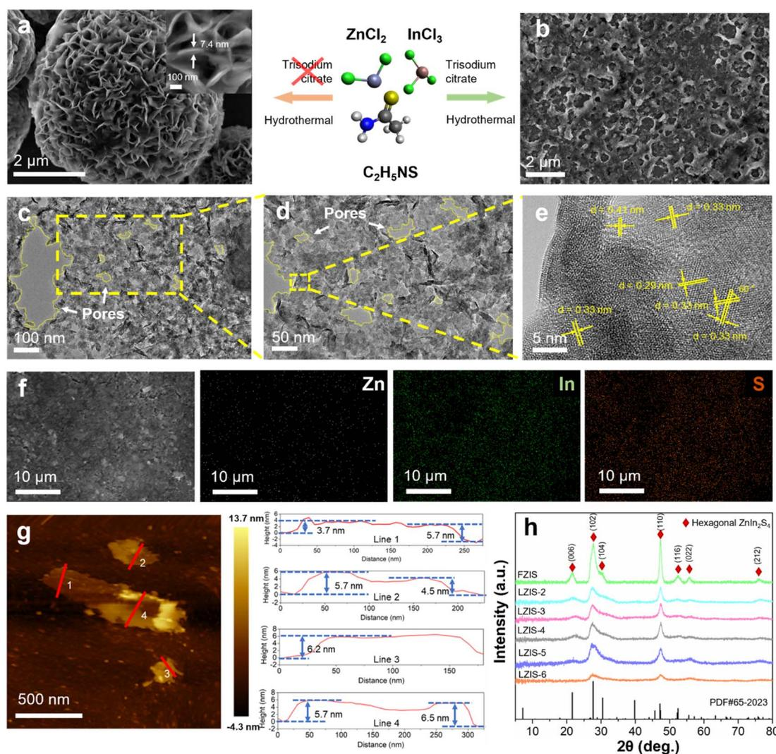
Fig. 1 FESEM images of (a) pristine  $\text{ZnIn}_2\text{S}_4$  nanoflowers and (b) LZIS-4. The inset of (a) depicts the thickness of the pristine  $\text{ZnIn}_2\text{S}_4$  nanoflowers. (c and d) TEM and (e) HRTEM images of LZIS-4. (f) FESEM-EDX mapping images of LZIS-4, where white, green and red represent Zn, In and S, respectively. (g) AFM topographic image and the corresponding height profiles of LZIS-4. (h) XRD of the as-prepared  $\text{ZnIn}_2\text{S}_4$  samples.
