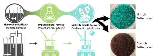
Lithium-ion battery black mass (LIBBM) processing through 3 Steps: EC-leach, phosphate impurity removal and Tutton's salt recovery of Ni and Co by fractional precipitation.
