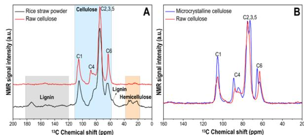
Fig. 4 SS-<sup>13</sup>C NMR (A) between rice straw powder and raw cellulose; (B) between commercially microcrystalline cellulose and raw cellulose.
