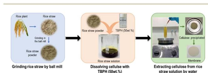
Fig. 1 A schematic diagram of lignocellulosic compound isolation.
