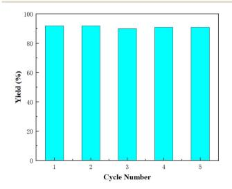
Fig. 2 Recyclability of catalyst L1-NiBr<sub>2</sub> for the coupling of CO<sub>2</sub> and 1a (1 mmol).
