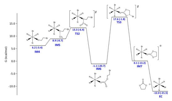
Fig. 4 Energy profile for the conversion from the  $CoN_4BrOCH_2CH_2Br$  intermediate (IM4) to the final product, ethylene carbonate (EC). The original L1-NiBr<sub>2</sub> catalyst was selected to be the zero-energy scale to stay consistent with Fig. 3. The relative Gibbs free energies and the relative electronic energies (in parentheses) in kcal  $mol^{-1}$  are labelled.
