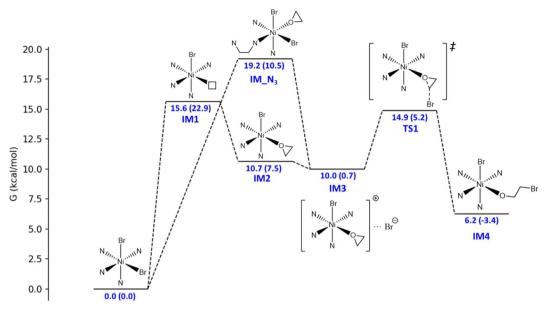
Fig. 3 Energy profile for the binding of the L1-NiBr<sub>2</sub> catalyst with the ethylene oxide substrate, followed by the nucleophilic ring opening process. The relative Gibbs free energies and the relative electronic energies (in parentheses) in kcal mol<sup>-1</sup> are labelled.
