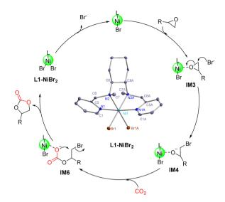
Scheme 3 A proposed mechanism for the cycloaddition reaction catalyzed by L1-NiBr<sub>2</sub>.
