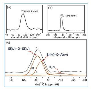
Fig. 8 (a)  $^{29}$ Si MAS NMR of alumino-silicate materials. (b)  $^{27}$ Al MAS NMR of alumino-silicate materials. (c) The  $^{17}$ O MAS NMR spectrum of the alumino-silicate materials is designated as p and the deconvoluted spectra, labelled as m, n, and k.
